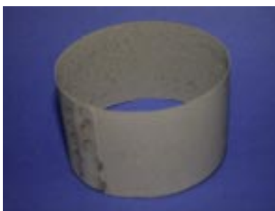
Figure 9. Resistance spot welded cylinder of porous sintered Ni-Cr-2xAl-Fe powder.
