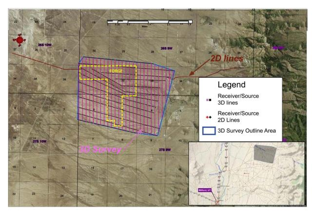
Map of the layout of the 3D seismic survey 2D seismic lines. The 3D survey is contained within the blue lines covering  $^{18}$  km<sup>2</sup> (7 mi<sup>2</sup>).
