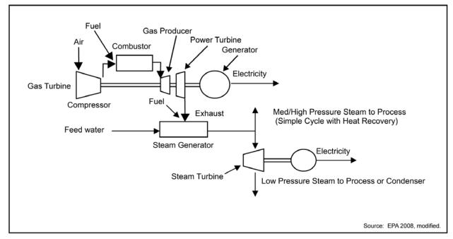
Figure 2-3. Generic representation of a CHP plant as would be deployed by Seattle Steam.
