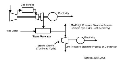
Figure 2. Generic representation of a CHP plant as would be deployed by Seattle Steam.
