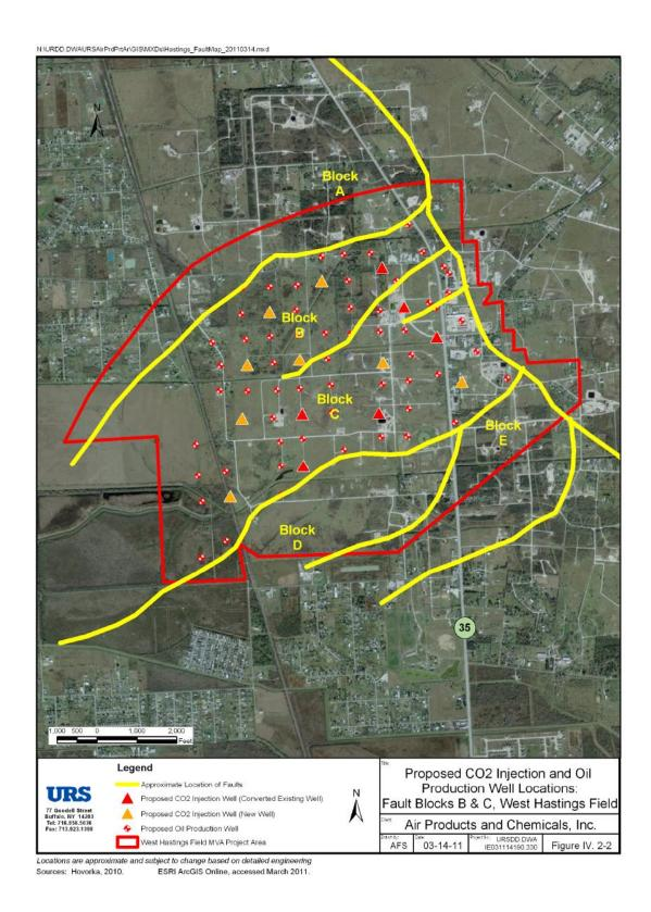
$\begin{tabular}{ll} \textbf{Figure IV.2-2.} & Proposed $CO_2$ Injection and Oil Well Locations in Fault Blocks $B$ and $C$ - West Hastings Field \\ \end{tabular}$
