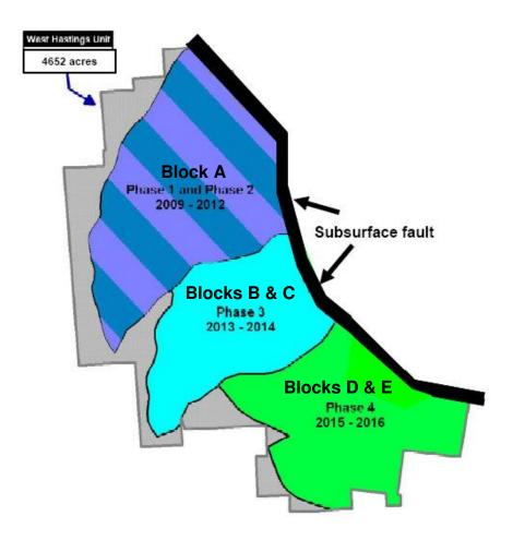
**Figure IV.2-1.** Proposed Phased Implementation Schedule for CO<sub>2</sub> Injection into the West Hastings Field.
