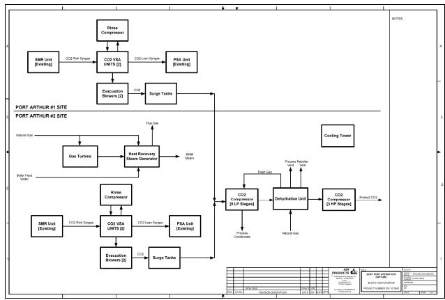
Figure II.2-2. Conceptual Process Flow Diagram for the CO<sub>2</sub> Capture Process
