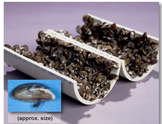
The small zebra mussels densely colonize inside cooling water intake pipes of power plants thus leading to significant power outages and expense.
