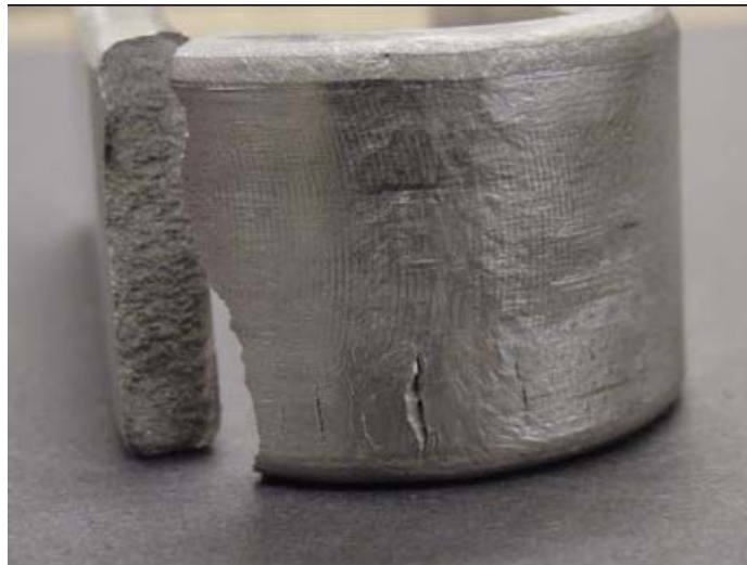
Figure 9: PWHT side-bend test specimen – failed in Nimonic 263 base metal, cracking also in root area of weld metal
