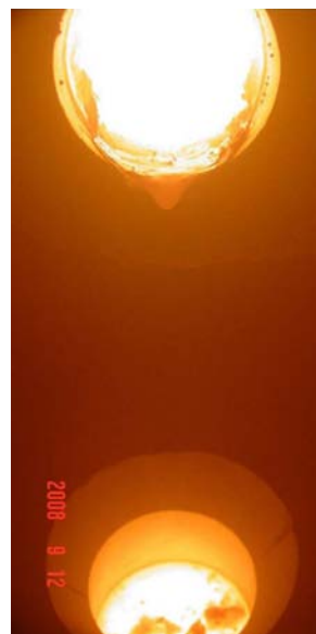
Casting a sample of one superalloy candidate from the melt crucible (top) into a mold designed to stay below 550°C (at right) to simulate the slow cooling that occurs for large castings.
