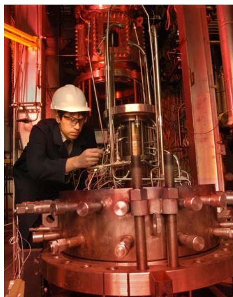
NETL engineer inspects the CCADS installation in the SimVal rig section.
