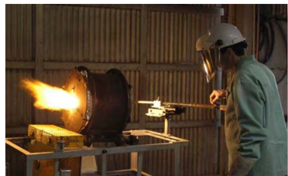
Laboratory test of refractory performance under extreme operating conditions.
