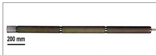
Photograph of a Pall Corporation iron aluminide hot-gas filter. These filters, made from an ORNL-developed alloy, give excellent performance in coal gasification plants. Over 2,000 are now in use, some for over six years.
