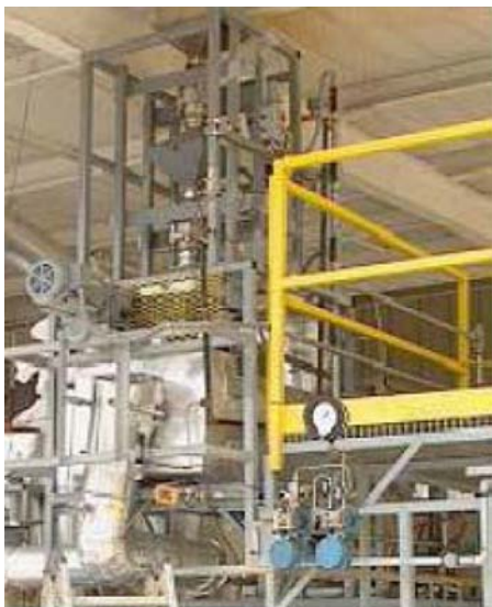
Pilot plant pyrolysis unit with biomass feedstock system.
