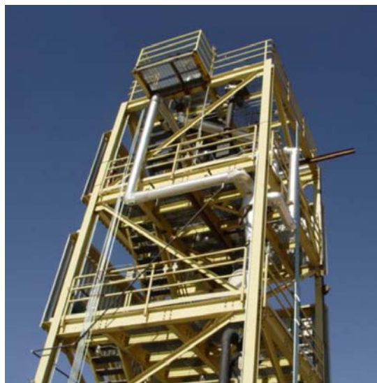
Process Development Unit at WRI Advanced Technology Center provides pilot-scale testing of advanced pollutant removal techniques.
