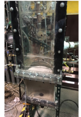
Semi-circular fluidized bed with side jets.
