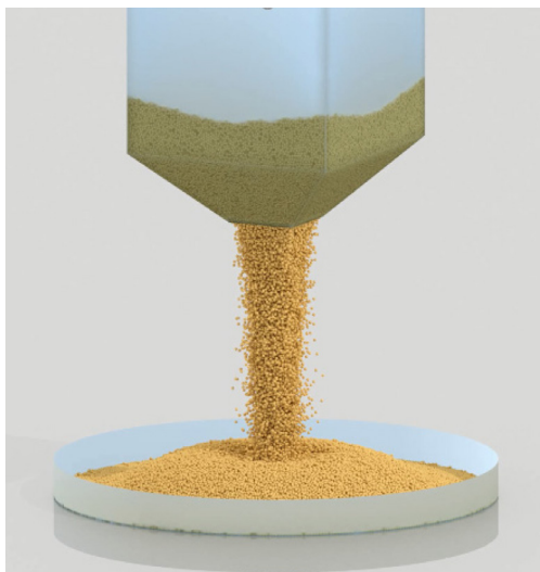
MFIX-DEM simulation of granular solids discharge from a hopper.
