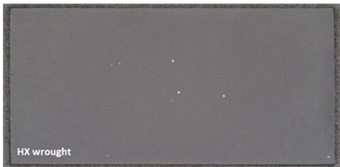
No spallation for wrought HX 4x100 hours at 950 °C.
