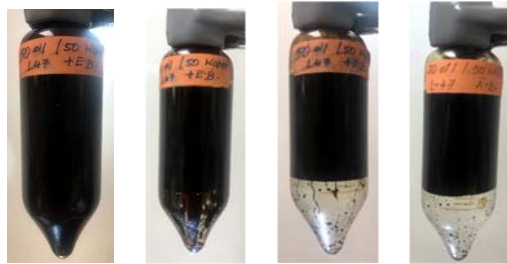
(a) 0.25 hr (b) 0.5 hr (c) 2 hr (d) 4 hr Figure 59 Bottle test of L-47 emulsion with emulsion breaker.
