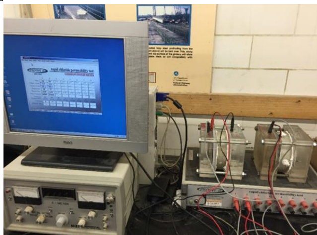
Figure 1: An electro-migration test unit.
