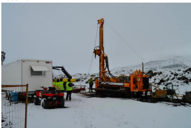
Figure 1: Wireline diamond drilling rig at the CarbFix injection site in October 2014. Photo: M. Stute.
