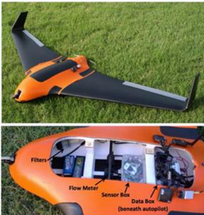
Figure 1: The Skywalker X8 platform will act as the UAV for sensor testing at the FWU site
