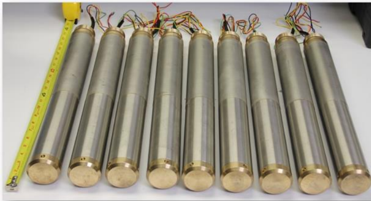
Figure 1: GPUSA's seismic source modules, like those shown here, are capable of both cross-well and vertical monitoring.
