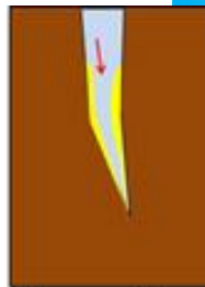
Uniform carbonate layer along fracture surface
