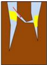
New fractures due to volume expansion brought by carbonation
