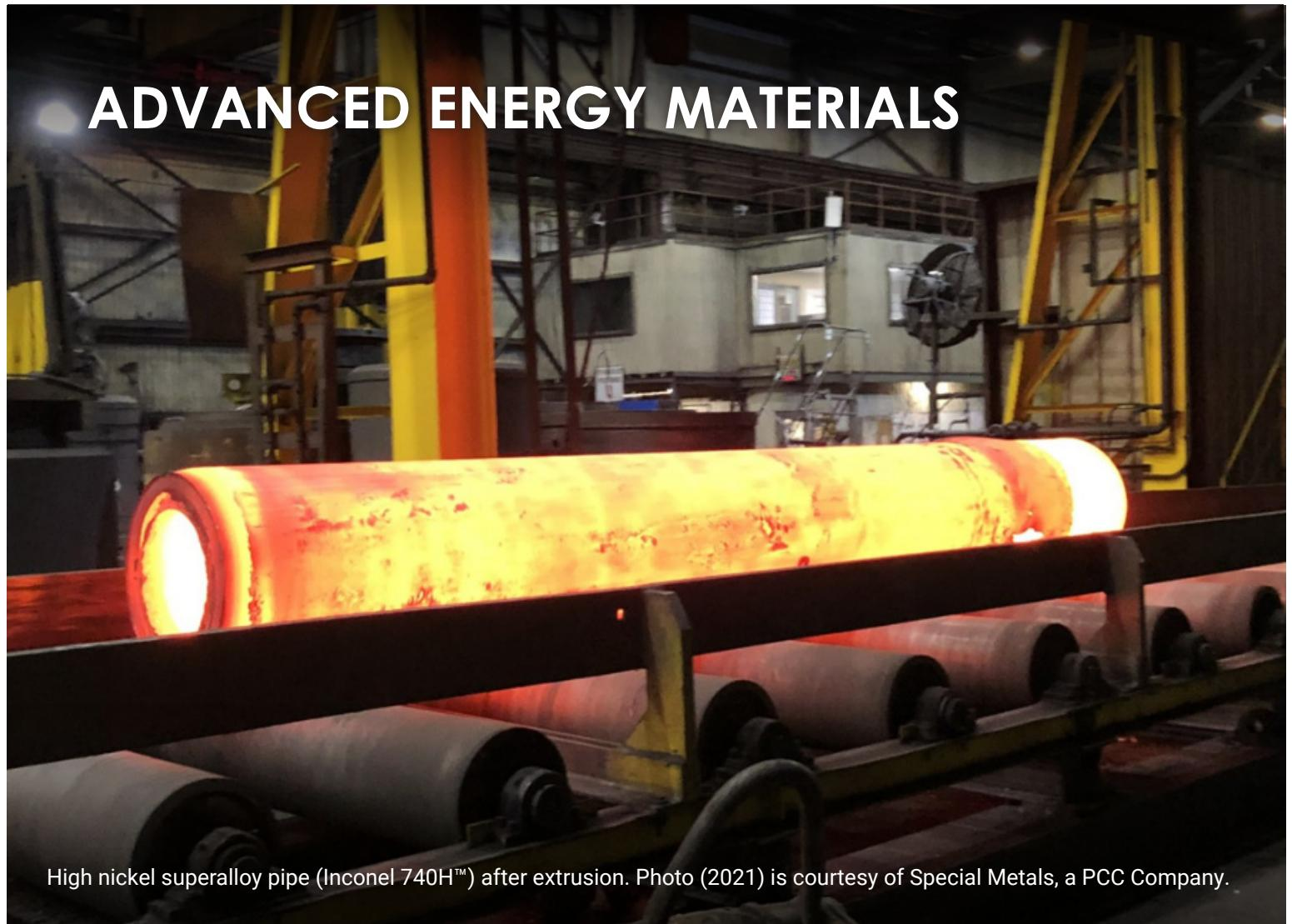
High nickel superalloy pipe (Inconel 740H™) after extrusion. Photo (2021) is courtesy of Special Metals, a PCC Company.
