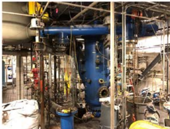
Figure 3: Pilot-scale U-GAS feed system.
