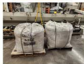
Figure 6 Pelletized fuel feed used for C&D waste-to-hydrogen gasification trials
