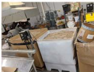
Figure 5 Hammermilled C&D waste "fluff," preparing to be pelletized
