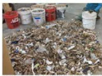
Figure 3 C&D waste shear-shredded to 2" minus and screened for metals, preparing for hammermilling
