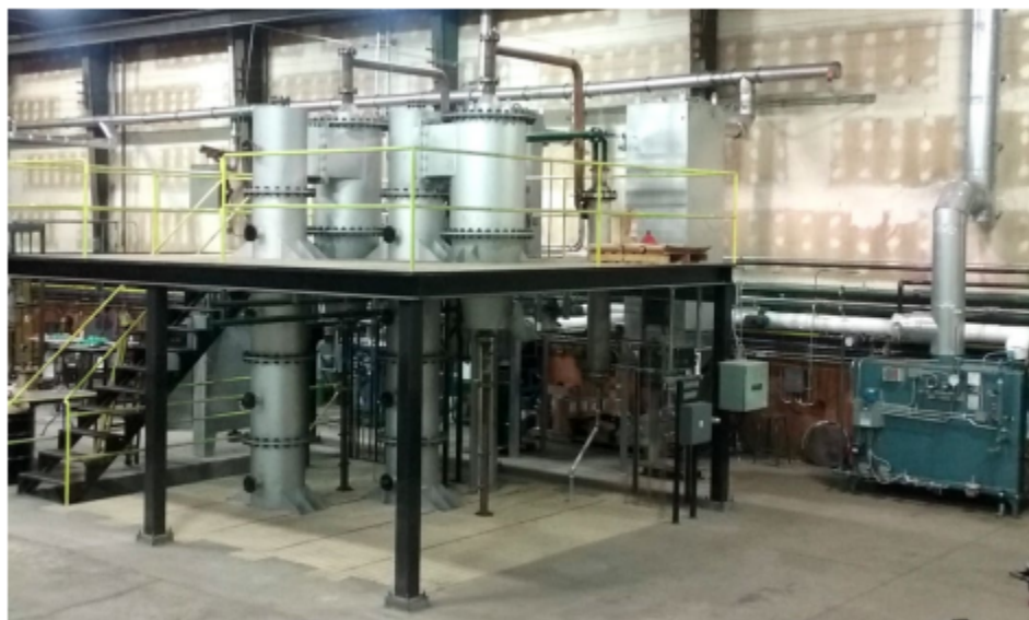
Figure 6: University of Utah dual fluidized bed process development unit.
