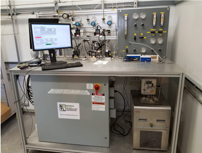
A test apparatus designed and built by NETL to measure gas permeance for CO 2 separation membranes at the National Carbon Capture Center in Wilsonville, Alabama.
