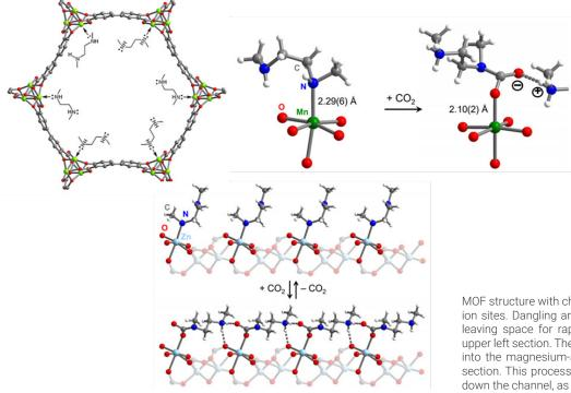
MOF structure with channels that are lined by open magnesium ion sites. Dangling amines coat the periphery of the channels, leaving space for rapid diffusion of CO<sub>2</sub>, as illustrated in the upper left section. The capture process involves insertion of CO. into the magnesium-amine bond as shown in the upper right section. This process is then replicated - or stepped - moving down the channel, as shown in the bottom part of the Figure.
