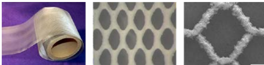
Figure 1: Microlith mesh coated with sorbent—cell opening 600 μm.
