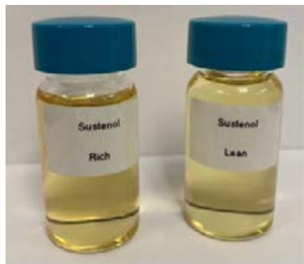
Figure 1: (left) Sustenol™ solvent samples; (right) superior CO 2 capture performance of Sustenol over 30wt.% MEA in 1 TPD pilot unit.
