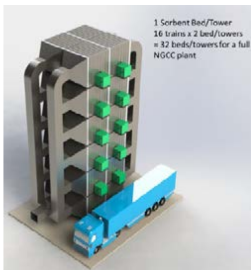
Figure 3: Single sorbent bed/tower with 24 individual sorbent modules (two each in series in flue gas flow direction and 12 such two-in-series modules in parallel). Bed height is 72 feet.
