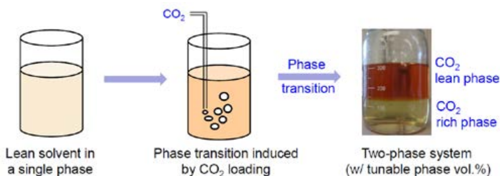
Figure 1: Phase transition behavior of a biphasic solvent.
