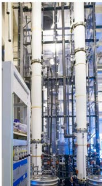
Figure 5: SRI's large bench-scale integrated absorber-regenerator system (gas flow rates up to 600 standard liters per minute).
