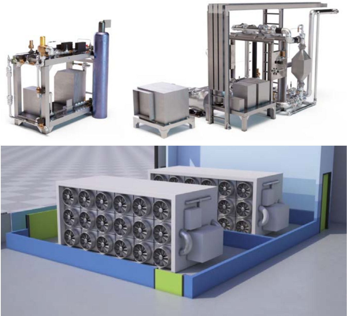
Figure 1: Renderings of the three scales of testing at the NETL DAC Center: Material Scale (top-left), Module Scale (top-right) and Prototype Scale (bottom).
