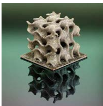
Figure 2: TPMS structure printed using metal AM at LLNL.
