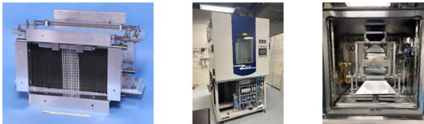
Figure 1: Left: Image of a DAC contactor, shown here with 50 plate pairs, 10 coated with 100 g of RTI sorbent on each plate. Center: Exterior of the test chamber for long-term testing of contactor modules. Right: Interior of the test chamber.
