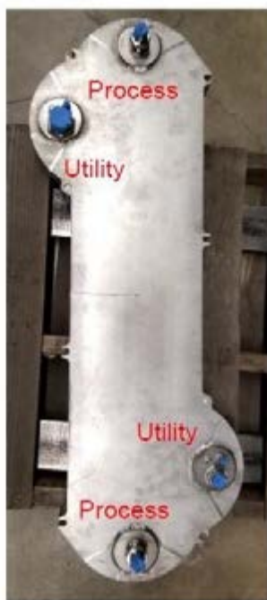
Figure 3: Illustration of ITAPS microchannel heat exchanger units/reactors. Highly efficient, low-cost heat exchanger.
