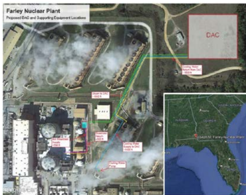
Figure 1: Satellite image of the Farley Nuclear Plant, including proposed locations for DAC site and key resources onsite. Inset: Geographic location of the Farley Nuclear Plant, the proposed host site for this project.
