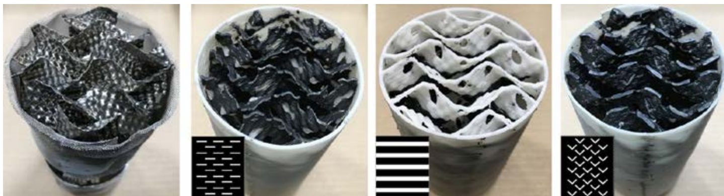
Figure 3: 250Y-type packing comparison with different dynamic design patterns (left to right) SS, DP-1, DP-2, DP-3.
