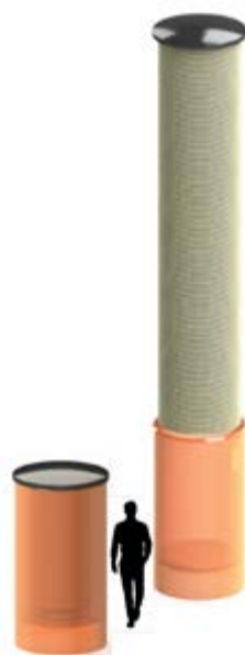
Figure 1: Carbon Tree in capture (right) and regeneration modes (left).
