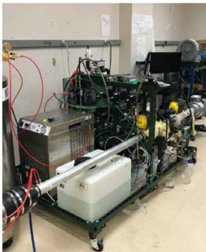
Figure 1: GT's laboratory-scale system used to test and validate monolith adsorption performance, desorption performance, and cycle times.
