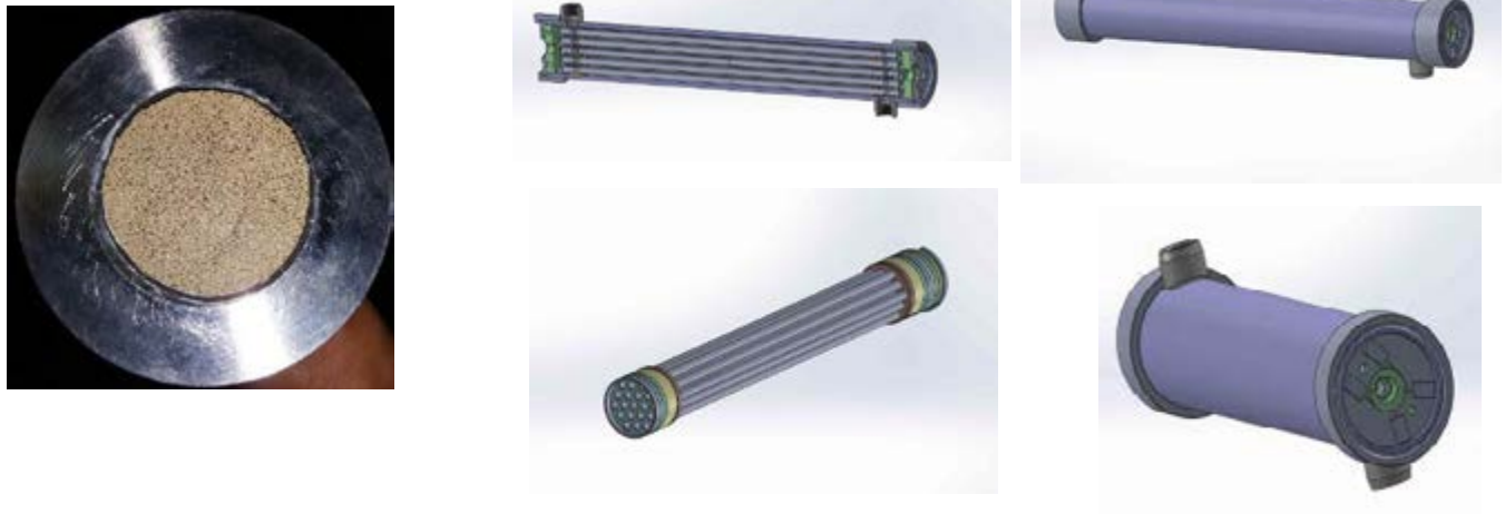
Figure 4: Potted module cross-section (left-most); new tube sheet module design (right).
