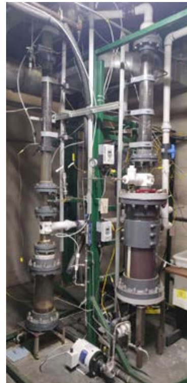
Figure 2: Completed bench-scale UK compact absorber.
