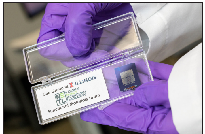
A functional memristor computer memory device fabricated in a collaborative project between NETL and the University of Illinois at Urbana-Champaign. The atomically thin dielectric carbon film used as the switching media in this device is made from domestically sourced coal and outperforms the metal oxide films typically used for this application.
