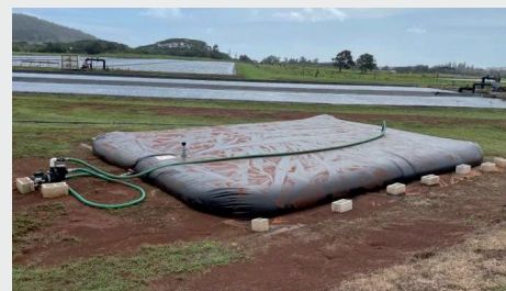
Carbonated Media Bladder Tank
