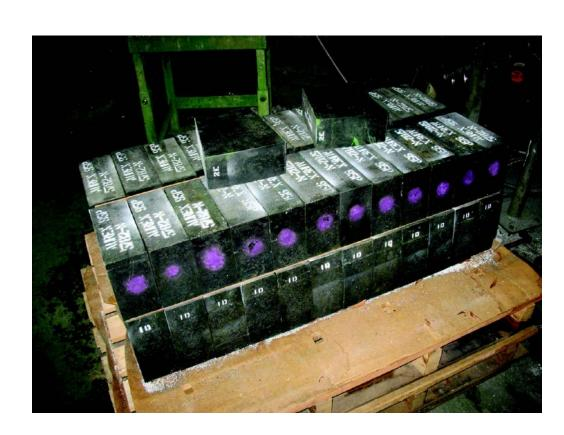
NETL developed refractory brick doubled refractory service life. Licensed to Harbison-Walker and commercially produced as Aurex 95P. Used in nearly every slagging gasifier worldwide.
