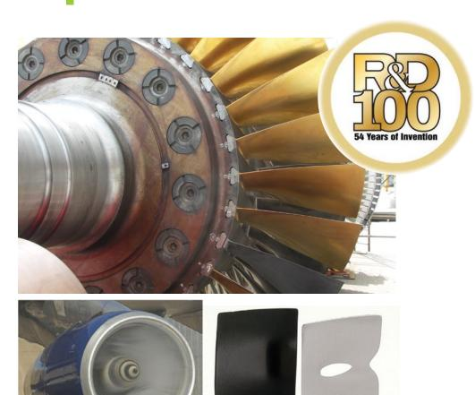
BlackGold<sup>®</sup>, an erosionresistant nanocoating for gas turbines, developed with MDS Coatings and partners Delta and Calpine.
