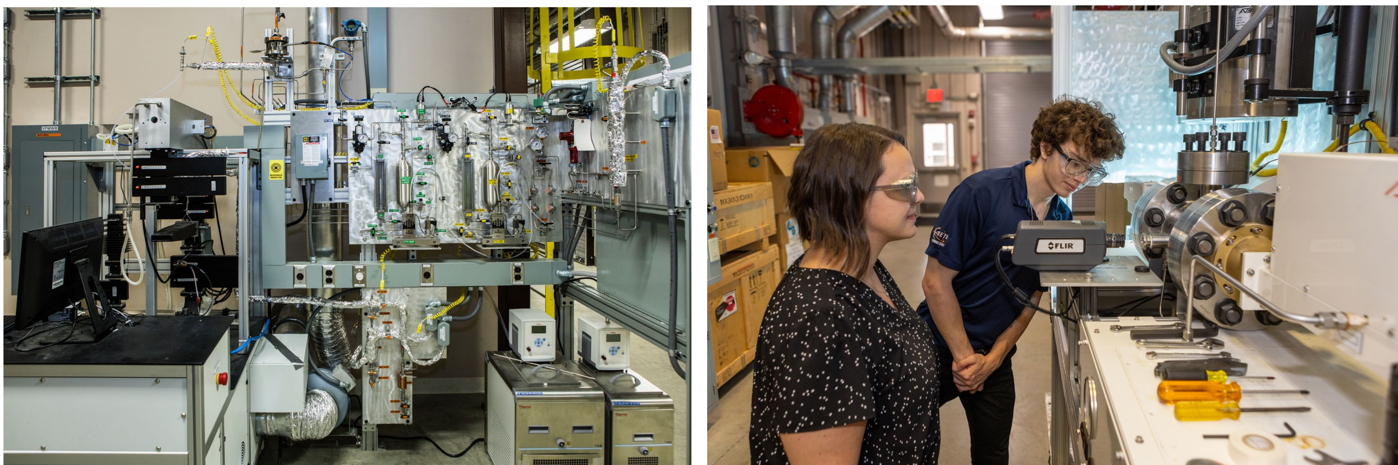
Left, a continuous variable frequency microwave reactor (frequency 2-8 GHz, power 0.6kW). Right, high-pressure (36 bar) microwave reactor (2.45 GHz, and 3 kW).
