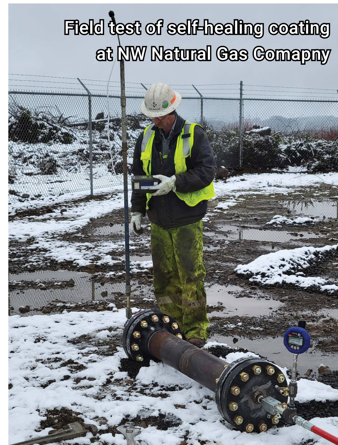
Field testing of a pipe with self-healing coating on interior surface at a NW Natural Gas Company site.
