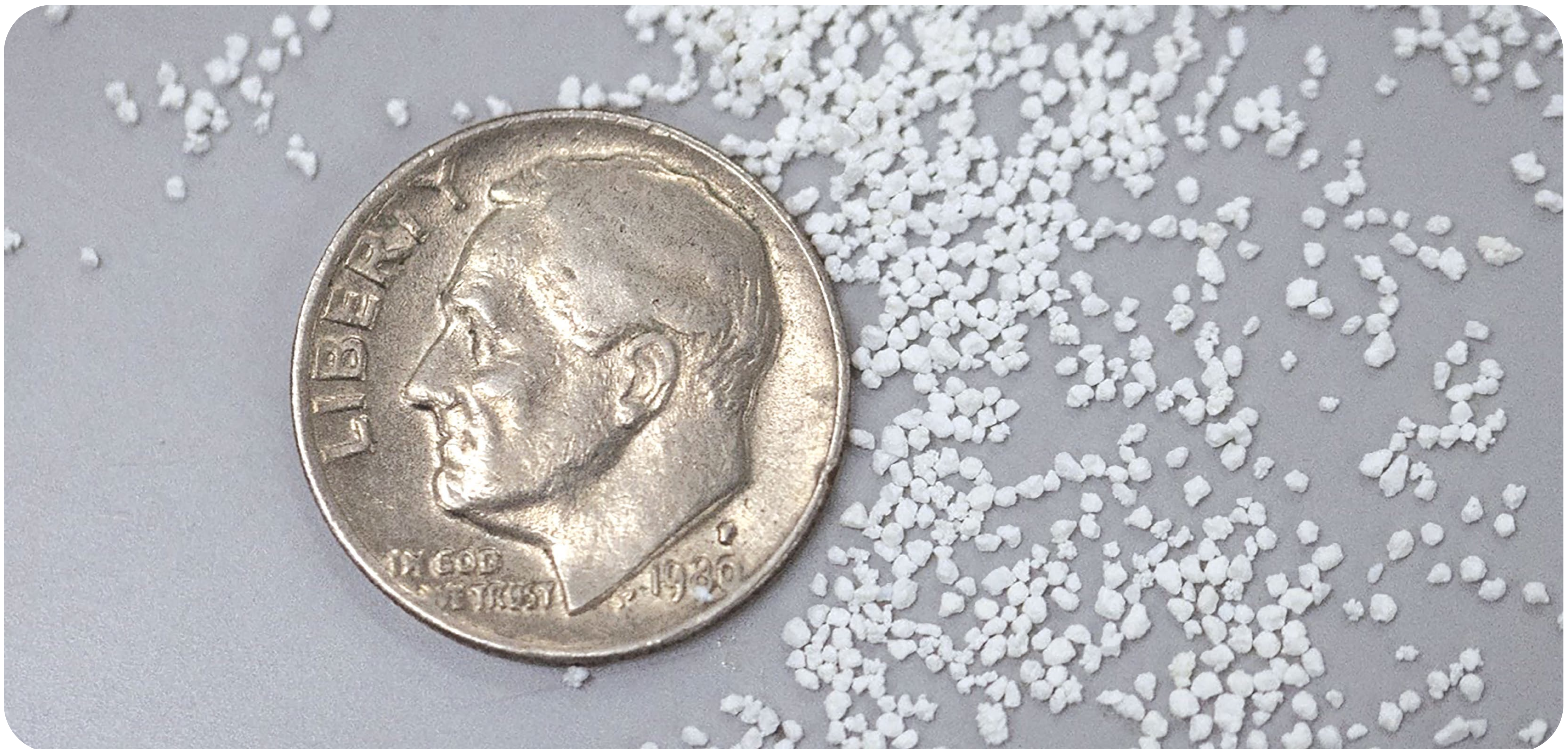
NETL's low-cost durable DAC sorbent with high selectivity and adsorption capacity for CO 2 .
