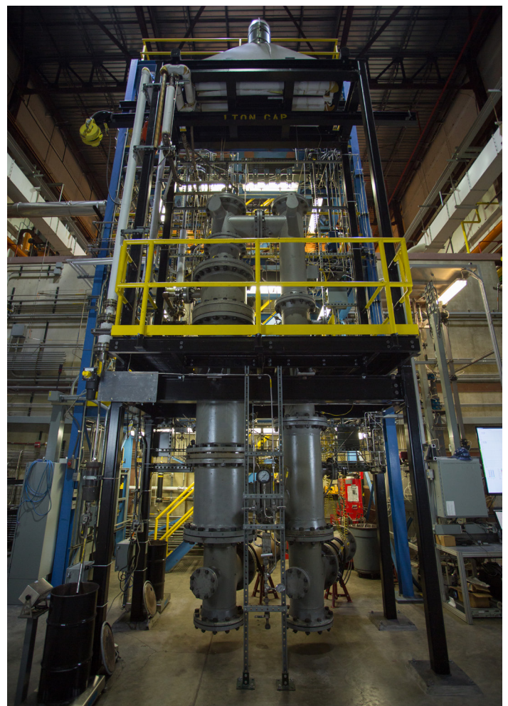
Figure 4. 50-kWth chemical looping reactor.
