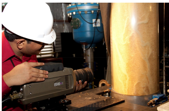
Figure 3. Researcher collecting high-speed video for particle tracking.
