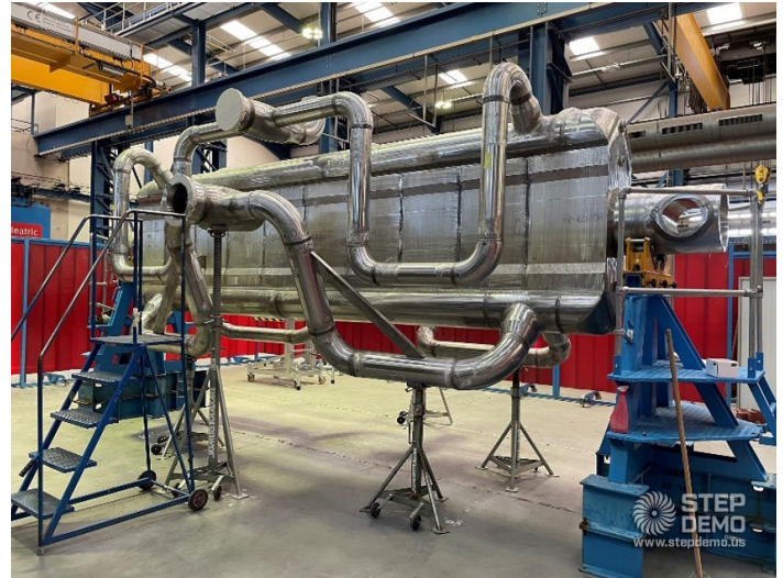
Figure 4. High Temperature Recuperator fabricated by Heatriac for the 10 MWe STEP Pilot Plant Test Facility
