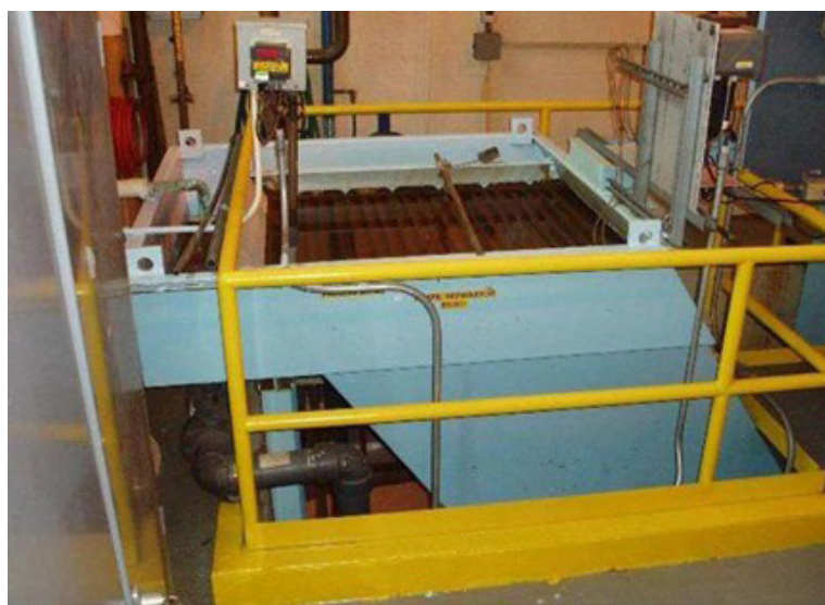
Photo 3.2.6.1: Pittsburgh plate separator.
