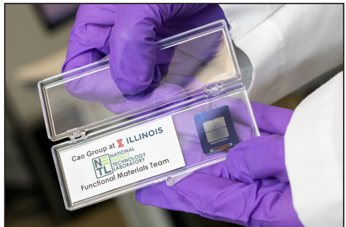
A functional memristor computer memory device fabricated in a collaborative project between NETL and the University of Illinois at Urbana-Champaign. The atomically thin dielectric carbon film used as the switching media in this device is made from domestically sourced coal and outperforms the metal oxide films typically used for this application.
