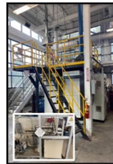
Pilot scale HAMR facility and high vacuum reduction setup (inset) for critical metals production
