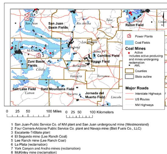
Location of coal fields, active and inactive mines, and coal burning power plants in the project area.
