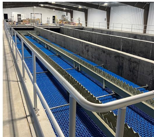
Internal view of the pilot-scale facility, which will simultaneously treat acid mine drainage and produce an enriched rare earth element and critical mineral concentrate.
