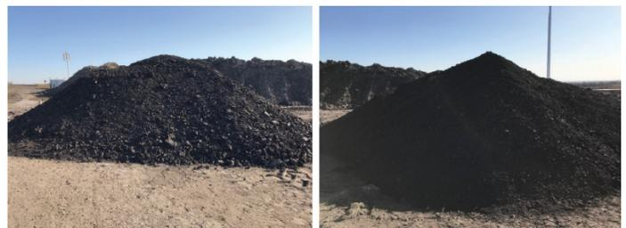
Coarse (left) and fines (right) coal piles extracted from Freedom Mine.
