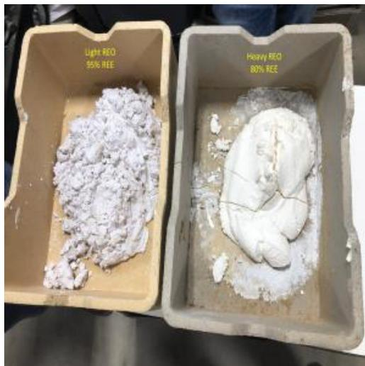
Recent Mixed Rare Earth Oxide (MREO) production at the A34 Facility which is operated jointly with the West Virginia Department of Environmental Protection. The A34 plant treats acid mine drainage for discharge to the headwaters of the Potomac River and produces these Light and Heavy MREO concentrates.
