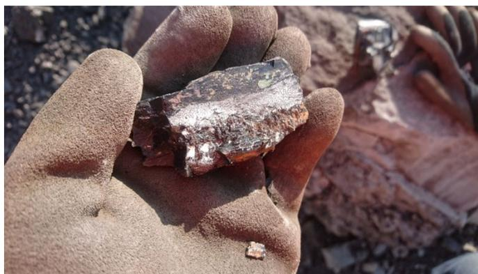
**A coal sample pulled from a location within the Greater Green River and Wind River Basins of WY & CO. This sample exhibits the uniqueness of coal-based materials for CORE-CM purposes. It has high-rank coal for utility in carbon ore products as well as clay materials hosting various rare earth elements and critical minerals.**
