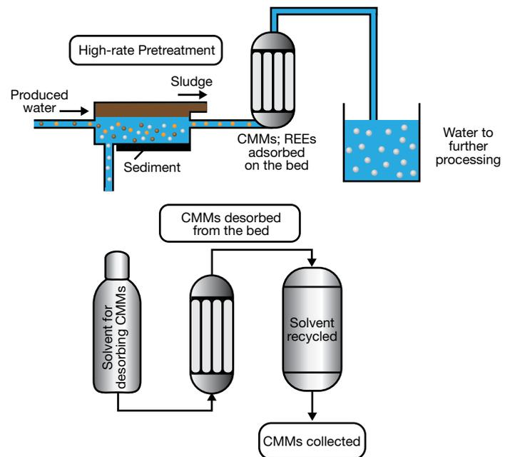
Diagram demonstrating low-cost environmentally friendly critical materials recovery from produced water.
