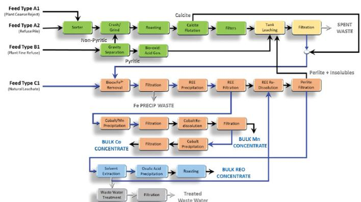
**Integrated process flowsheet showing the addition of innovative technologies implemented to enhance the economic extraction of REE, Sc, Co and Mn from pre-combustion bituminous coal-based sources.**
