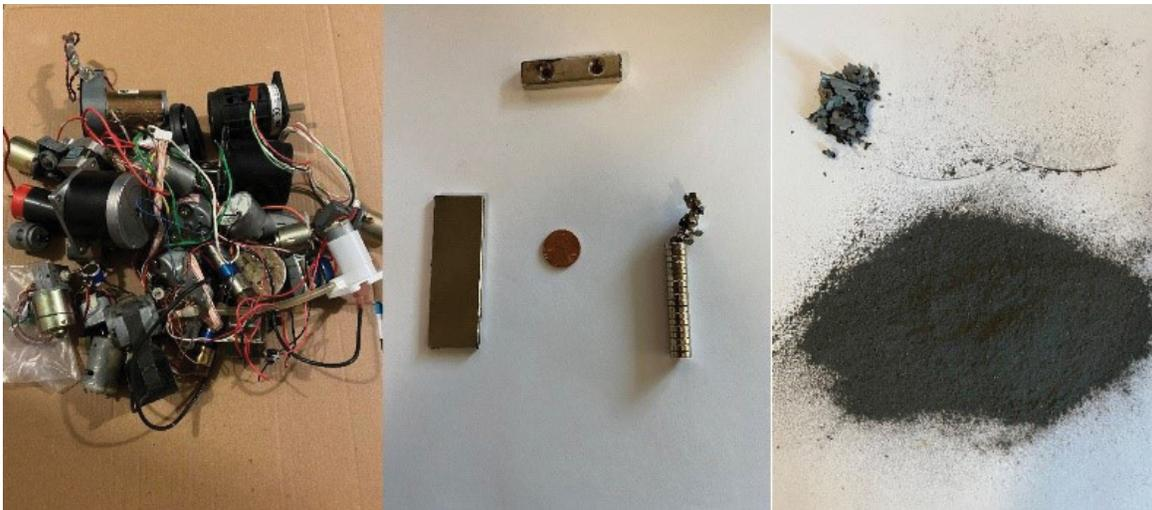
Left, used electric motors. Middle, used rare earth magnets. Right, recovered/recycled magnetic materials.
