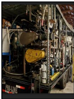
Hydrophobic-hydrophilic separation (HHS) process: Pilot scale facility
