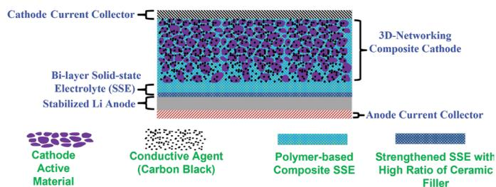
Schematic illustration of the proposed solid-state Li-ion batteries.
