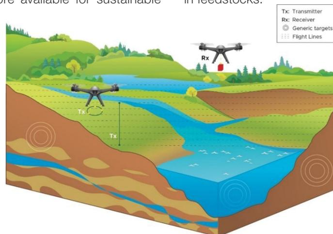
Schematic diagram illustrating both the fully airborne geometry with drone-based transmitter (Tx) and drone-based receiver(s) (Rx), and the semi-airborne geometry with a powerful ground-based transmitter and drone-based receiver(s).
