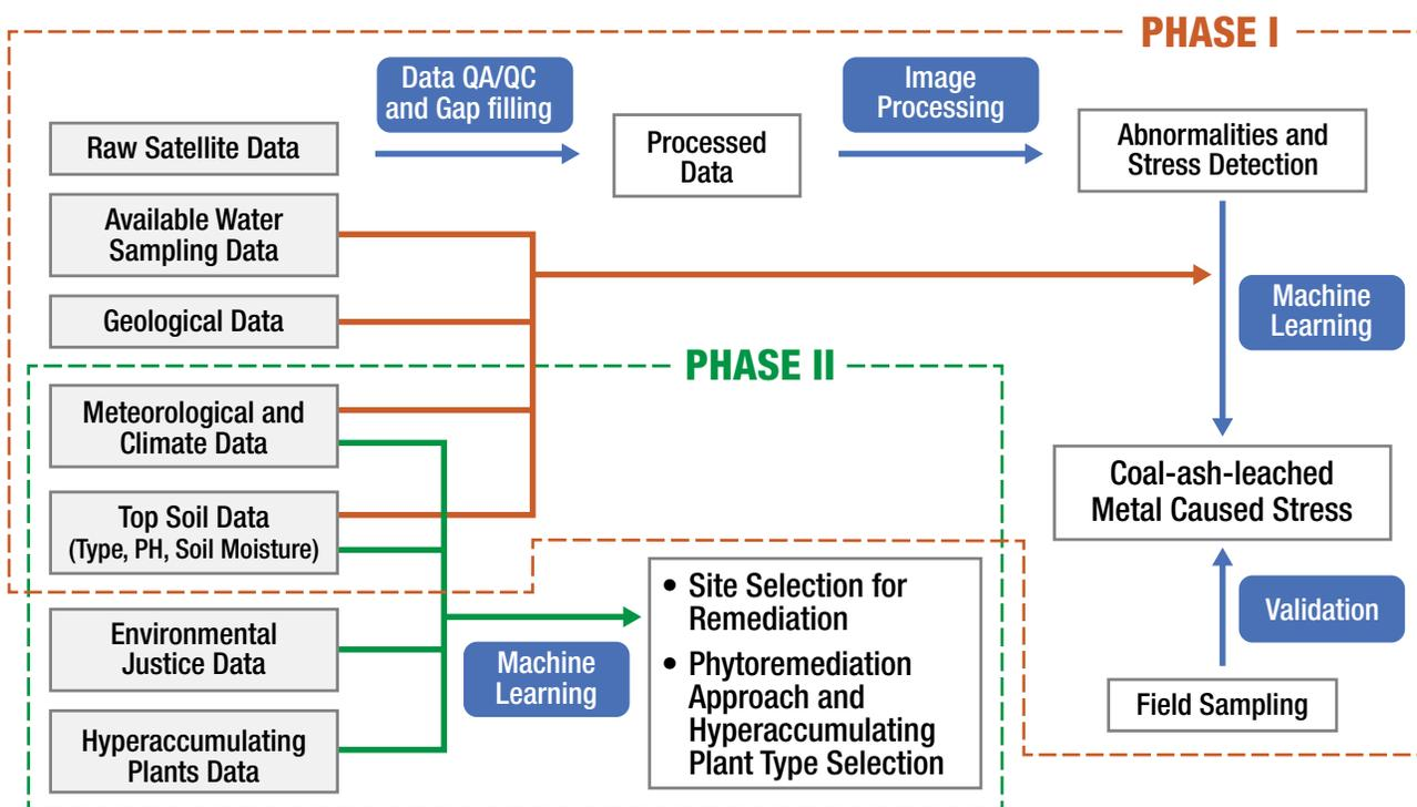
Diagram of phases 1 (identify potential leaching of metals from coal ash impoundments) and 2 (propose locally adaptable phytoextraction approaches to remediate contaminated regions) of the project.
