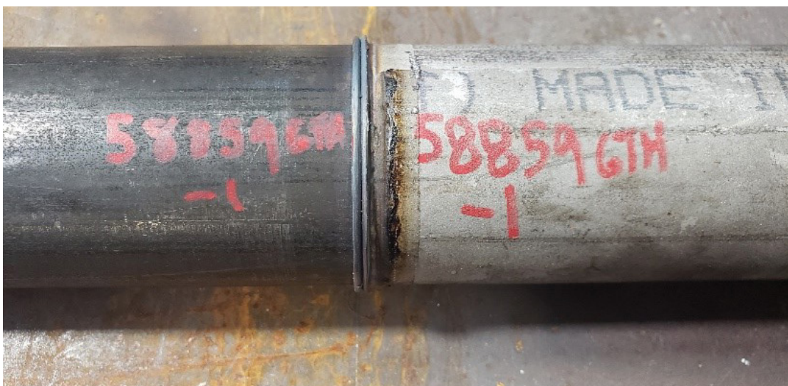
Rotary friction welded T91 to 304H tube.
