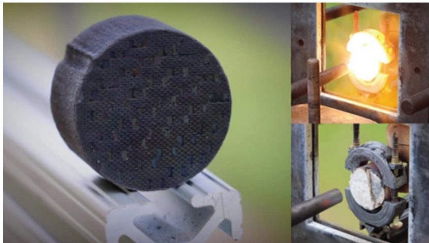
Flame exposure test of Ceramic Matrix Composite under an oxy-acetylene torch
