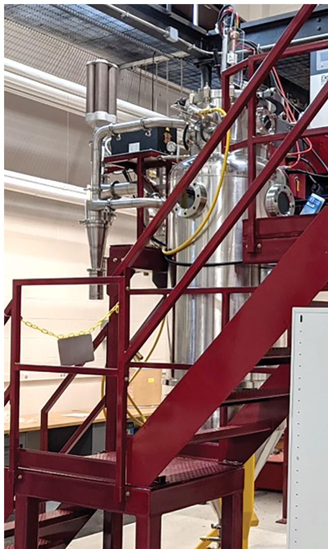
Spray deposition system at TTU for Cu-graphite nanocomposite manufacturing.
