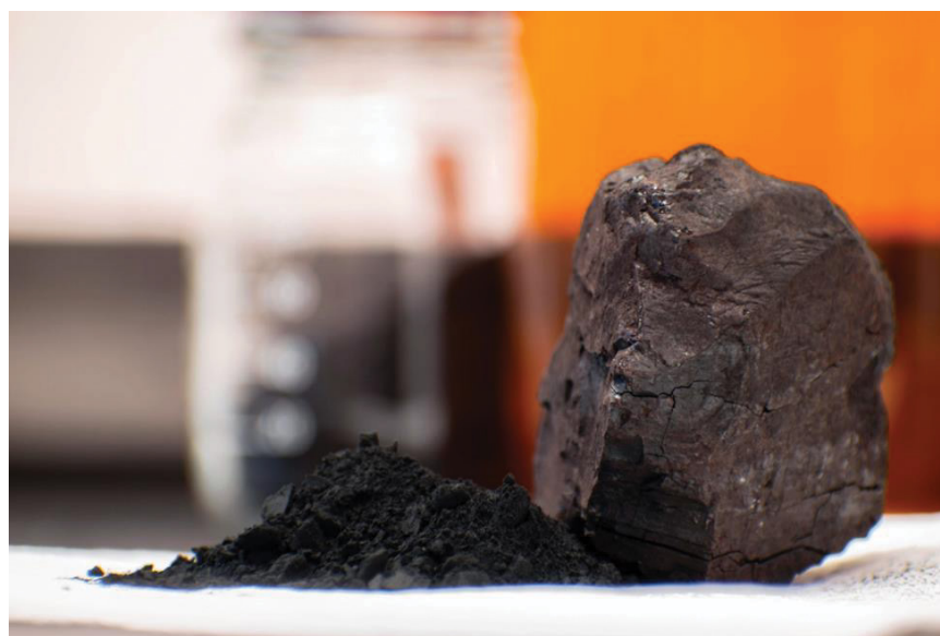
Powder River Basin coal, which will be used as a feedstock to produce GO, rGO, and graphene nanosheets.
