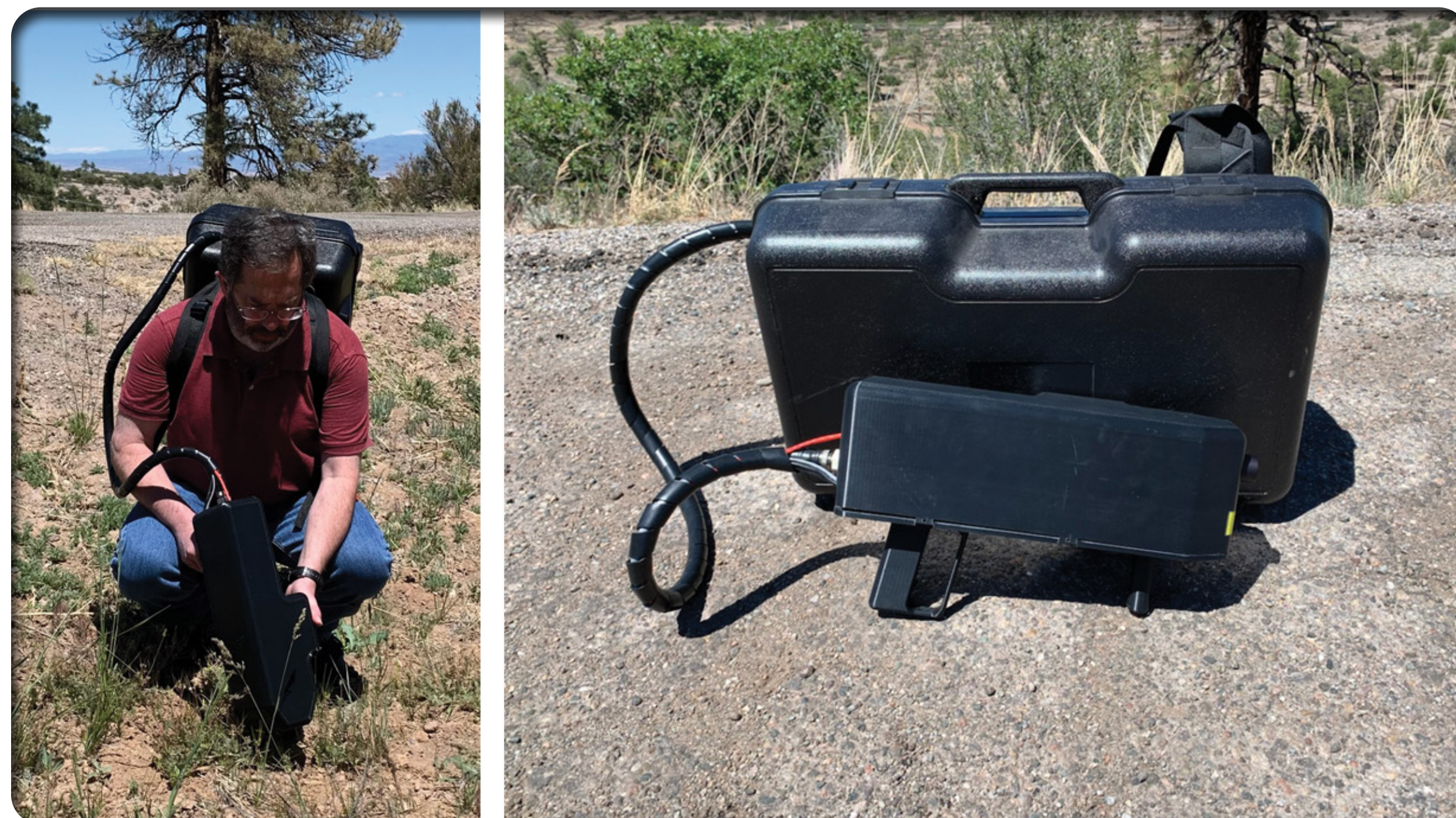
Left: The field-portable LIBS and Raman (backpack) prototype unit undergoing field testing. Right: Close-up of the field-portable unit.
