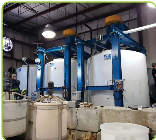
Three 3000-Gallon Bioreactors Used to Produce Two Gallons/Minute of Sulfuric Acid from Coal Pyrite at a Strength of Approximately 0.5M (One Bioreactor is a Feed Preparation Tank While the Remaining Two are Production Units Equipped with Denver Sub-Aeration Units Driven by 30 HP Motors and 8 Tons of Chilling Capacity)
