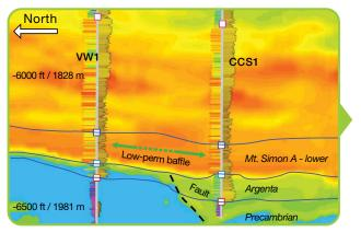
Visualization of **Cross Section Using Reflection of Seismic Porosity Inversion**
