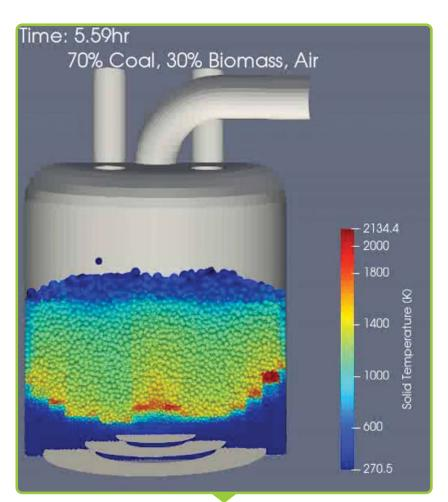
Gasifier Simulations with Mixed Coal-Biomass Feed
