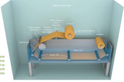
Roll-to-Roll Membrane Fabrication Machine Envisioned to Help Scale Up and Commercialize
