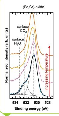
Ambient Pressure X-Ray Photoelectron Spectroscopy Was Used to Reveal Important Details of Alloy Degradation in Hot CO<sub>2</sub> by Analyzing the Reacting Alloy Surface in Situ
