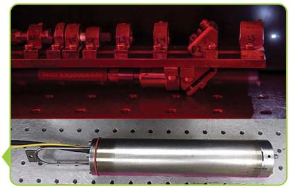
The complete downhole LIBS prototype sensor system was successfully deployed in a test well at the NETL-MGN site at 27-ft well depth (15 ft water depth). Measurements were performed on 14 days over a 20-day period. Results demonstrate the full system works in the target environment without serious complication, which raises the technology readiness level to 5: Lab/bench scale, similar system validation in relevant environment.
