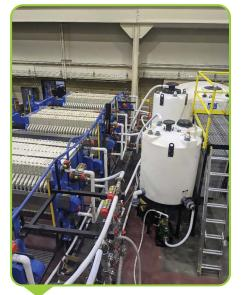
UND Coal Washing Systems Associated with the Coal Filter Presses
