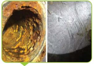
Typical Mic Damage to Spool (Left) vs. Dragx<sup>®</sup> Treated Spool After Six Months (Right)
