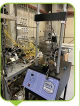
PCXT Anisotropic Permeability Chamber Measures Permeability in X, Y, and Z Directions PCXT Triaxial Stress Chamber Measures Mechanical Strength at Core Scale
