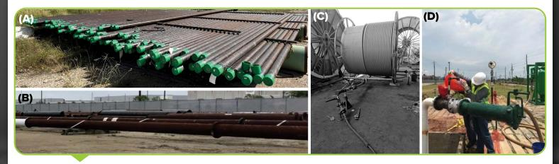
Test Applications of Dragx<sup>®</sup> Completed During This Effort Working With Different Industry Partners: (A) 8,000+ Feet of Casing Pipe, (B) 1,000+ Feet of Transport Pipe, (C) 10,000+ Feet of Coiled Tubing, (D) 1,000+ Feet of Wastewater Feed
