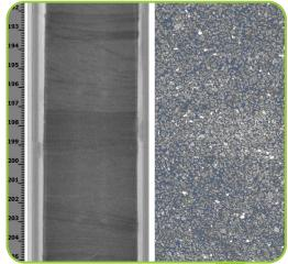
Pressure Core From Gulf of Mexico Showing Core-Scale Structure of Raw Sample (at Left) and High-Resolution X-Ray Ct Image of Completely Intact Pore-Scale Sediment/Hydrate Structure (at Right)
