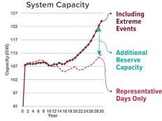
Traditional expansion planning could fail to include sufficient reserve capacity for extreme events. Inclusion of extreme events in the expansion planning models ensures sufficient reserves
