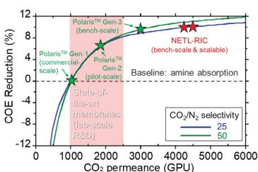
Cost of Electricity (COE) Cost Analysis Performed by NETL-RIC for Coal Flue Gas Decarbonization Using Membranes vs. Commercial Amine Absorption
