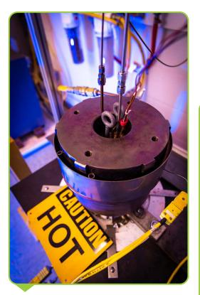
The Autoclave Reactor Is Used to Test Alloys in Flowing sCO<sub>2</sub> at Extremely High Temperatures and Pressures to Closely Simulate sCO<sub>2</sub> Power Cycle Environments
