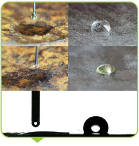
Image of Water Droplet on Untreated Pipeline (Left) vs. DragX<sup>®</sup> Treated Pipeline (Right).
