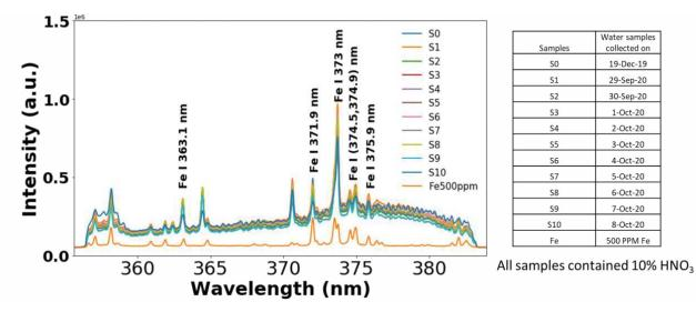
Averaged LIBS Spectra from NETL-Morgantown B19 Water Samples and 500 ppm Fe Calibration Sample
