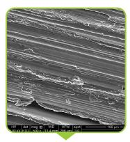
Steel Surface After Exposure to Non-Corrosive Cassh-1 Solvent
