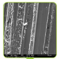
Carbon Steel Surface Before Exposure to Corrosive Solvent
