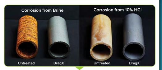
Images comparing untreated and DragX treated pipes corroded by brine (left) and 10% HCI (right).
