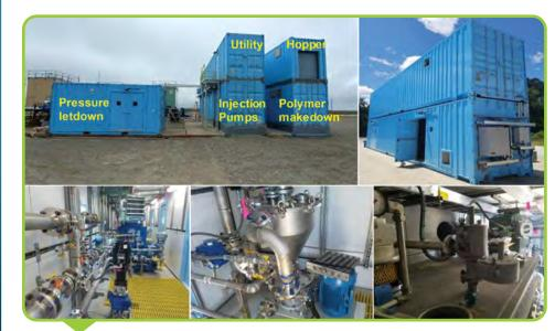
Polymer preparation equipment at NETL-supported field test on Alaska's North Slope.
