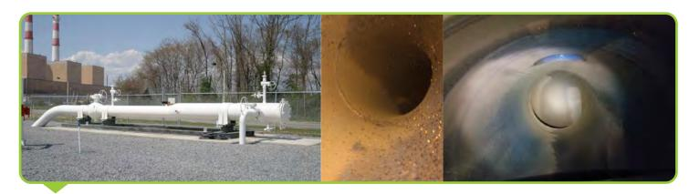
Representative image of test feeder line to simulate pig launcher (left), unprotected section (middle), and DragX treated section (right).
