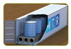
MTR's membrane-based capture system uses advanced membranes and compact, lowpressure-drop plate-and-frame modules contained in a modular unit that can be repeated in future commercial systems at low cost.
