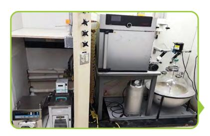
Acid digestion makes metals easier to separate by dissolving a coal ash sample into solution by adding acids and heating it until the metals break away from the other undesired materials. BMI successfully scaled up their acid digestion process to increase the concentration of mixed REE materials in solution and provided enough material for the RES facility.
