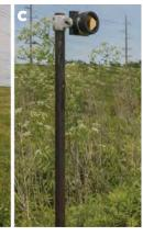
GreenLITE system. (a) layout showing chords from transceivers (T1 and T2) to reflectors, (b) transceiver installed, and (c) retroreflector installed at the IBDP site.
