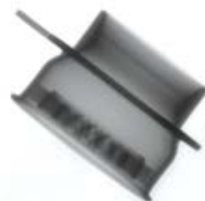
X-ray image of mixer part produced with RMM
