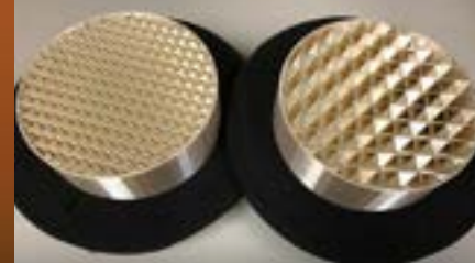
Packing with different cell densities, 3D printed at ORNL
