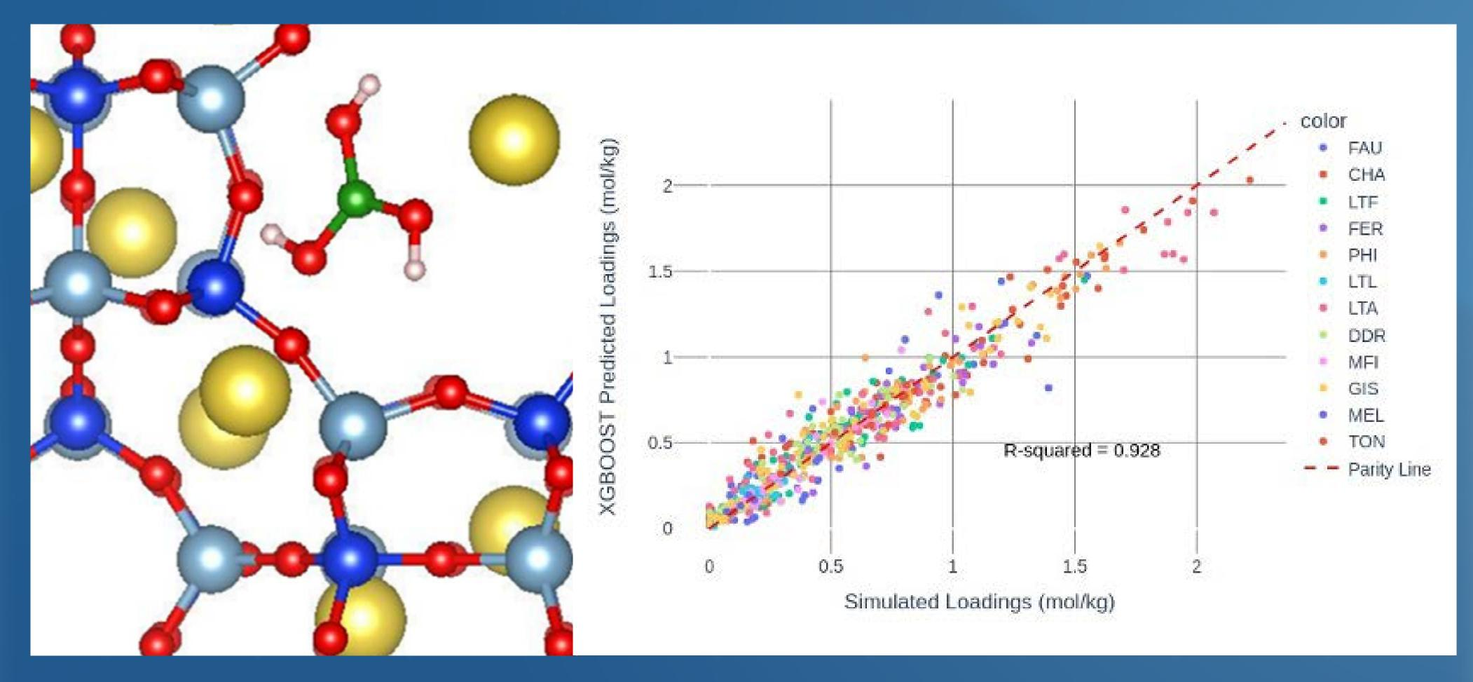
Machine learning methods were used to design zeolite sorbents optimized for boric acid uptake.
