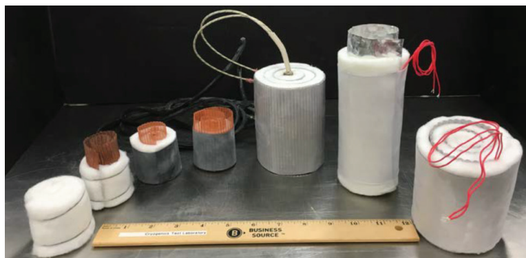
Various prototypes of CFC core modules (spiral configurations with different conductors).
