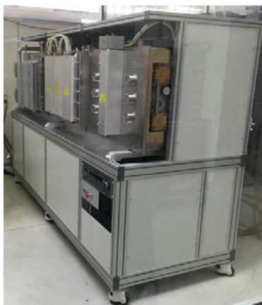
Fig. 2. TFE BVE3F magnetron sputtering system allowing for an up-scaled fabrication of Pd-alloy film.
