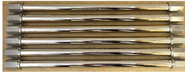
Fig. 5. Photograph showing six Pd–23%Ag/stainless steel composite membranes manufactured by SINTEF with permeable dimensions of 1 inch OD and 18 inch length.
