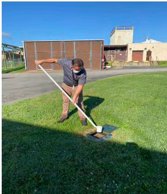
Photo 3.5.6.1: Storm water sampling at Out 002.
