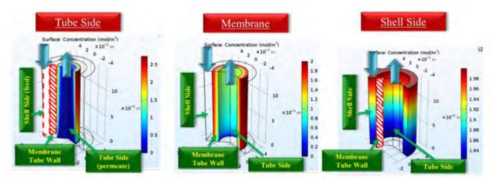
Figure 3: Single-tube membrane CFD gas concentration analysis.
