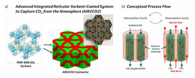
Figure 1: (a) Sorbent-coated contactor design showing sorbent-integrated channels (green) and hot air channels for desorption (red). (b) Conceptual process flow within alternating adsorption/desorption cycles.
