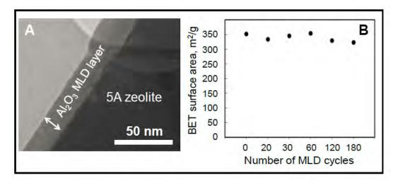
Figure 3: Characterization of MLD-modified 5A zeolite: (A) transmission electron microscopy (TEM) image of 5A zeolite with 60 cycles of aluminum oxide coating; (B) BET surface area of 5A zeolite with different cycles of MLD.
