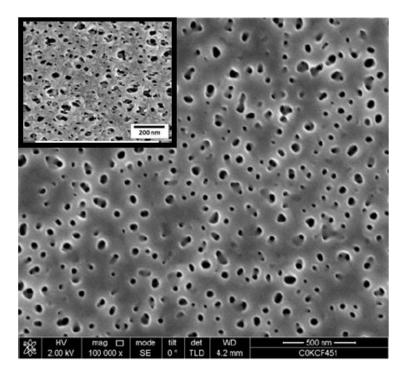
Figure 2: Top surface of a BCP1 support membrane. The inset is a conventional support.
