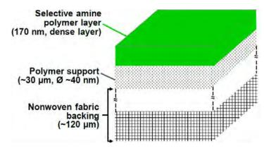
Figure 2: Schematic of the thin-film composite membrane.
