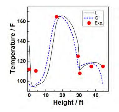
Figure 2: Absorber temperature profile (solid lines indicate model predictions for liquid and gas, experimental data in dots).
