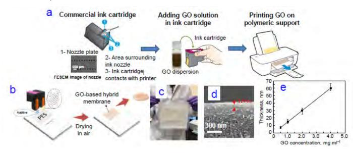
Figure 3: (a) Schematics of GO membrane fabrication by inkjet printing; (b) GO-based membrane preparation by printing from two cartridges containing GO ink and additives; (c) a picture of a printed GO membrane (15 cm × 15 cm); (d) cross-sectional SEM of the membrane; (e) dependence of membrane thickness on GO ink concentration.
