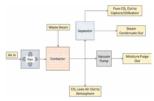
Figure 2: Block flow diagram of DAC system.
