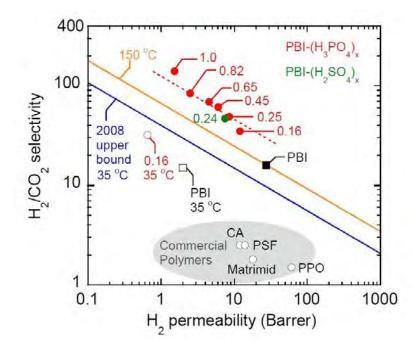
Figure 1: Pure-gas H<sub>2</sub>/CO<sub>2</sub> separation performance of PBI-(H<sub>3</sub>PO<sub>4</sub>)<sub>x</sub> (x = 0.16-1.0) and PBI-(H<sub>2</sub>SO<sub>4</sub>)<sub>0.24</sub> at 150°C versus Robeson's upper bound at 35°C and 150°C.
