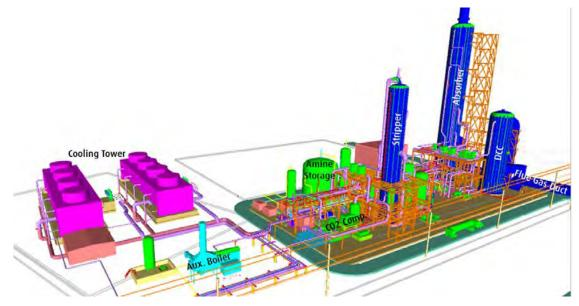
Figure 2: 3D layout of CO<sub>2</sub> capture plant.
