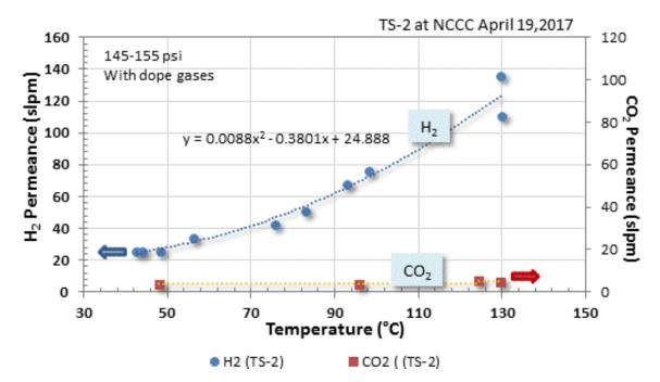
Figure 6: Measured H<sub>2</sub> and CO<sub>2</sub> permeances for the Gen-2 module at varying temperatures under a pressure differential of 145–155 psi.
