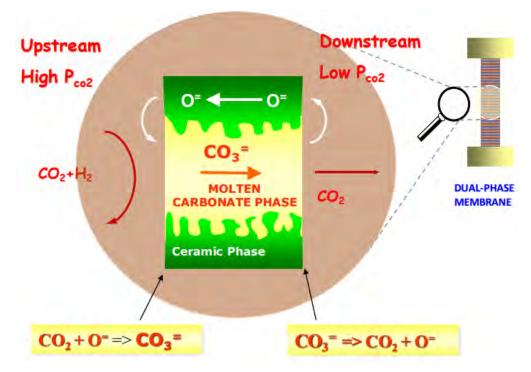
Figure 4: CO<sub>2</sub> separation mechanism in CCDP membrane.
