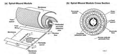
Figure 3: Schematic diagram of a spiral-wound membrane module.
