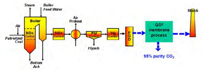
Figure 4: Process flow diagram for the proposed  $GO^2$  process for  $CO_2$  capture.
