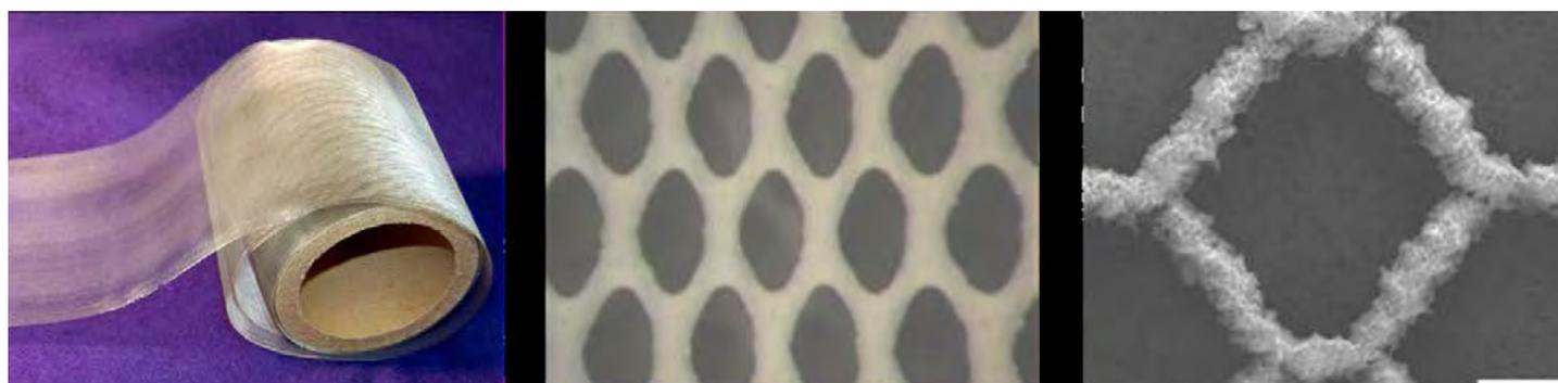
Figure 1: Microlith® mesh coated with sorbent.
