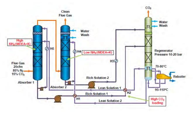
Figure 1: Conceptual process flow diagram for the A-MSP.
