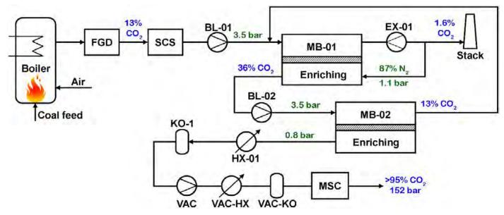
Figure 2: Process concept for two-stage membrane system. Initialisms: FGD = flue gas desulfurization; SCS = SO<sub>2</sub> caustic scrubber; BL = blower; MB = membrane; EX = turbo expander; HX = heat exchanger; KO = knockout; VAC = vacuum pump; MSC = multi-stage compressor.
