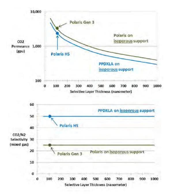
Figure 3: (a) Mixed-gas CO₂ permeance and (b) CO₂/N₂ selectivity as a function of selective layer thickness for Polaris<sup>™</sup> and PPDXLA on an isoporous support.
