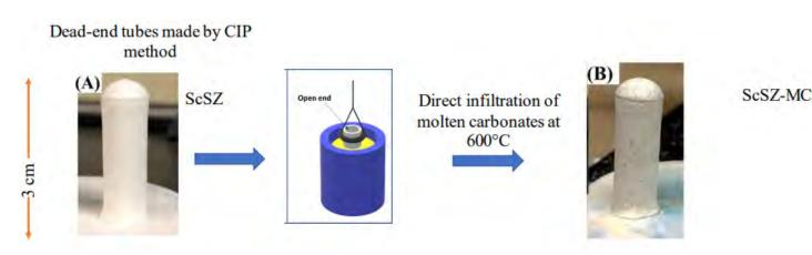
Figure 6: Sc-doped ZrO<sub>2</sub>(ScSZ)—(52/48 Li/Na)<sub>2</sub>CO<sub>3</sub>(MC).
