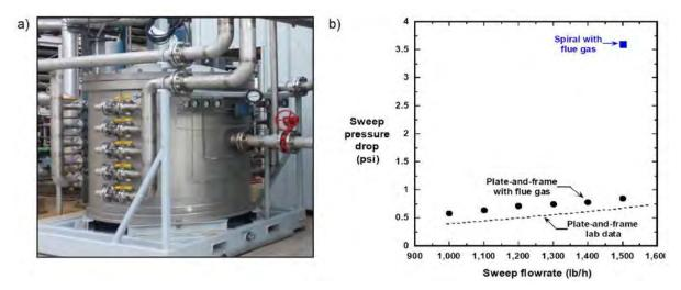
Figure 2: (a) Photo of the prototype planar module during testing at the NCCC, and (b) measured pressure drop in the module, compared to a conventional spiral-wound module.
