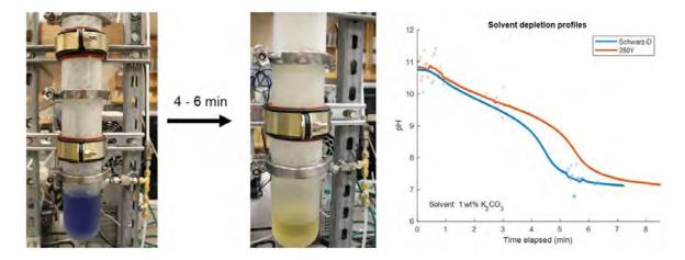
Figure 8: Colorimetric change of an aqueous K<sub>2</sub>CO<sub>3</sub> solvent using thymol blue as an indicator dye. pH evolution profiles for two absorber experiments using a TPMS Schwarz-D geometry and a conventional 250Y geometry.
