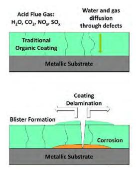
Figure 1: Mechanism for corrosion of coated metallic substrates.
