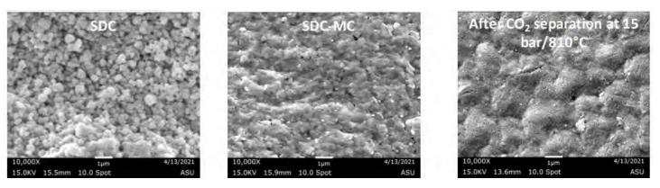
Figure 9: SEM images of high-pressure side of SDC membrane (left); SDC-MC (center); SDC-MC after high-pressure CO<sub>2</sub> permeation (right).
