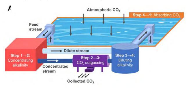
Figure 2. System schematic for ACS implementation. (A) Flow diagram indicating the three steps of the ACS: (1) concentration; (2) CO<sub>2</sub> extraction; (3) dilution and re-equilibration with air.
