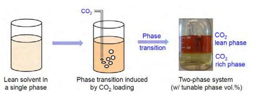
Figure 1: Phase transition behavior of a biphasic solvent.
