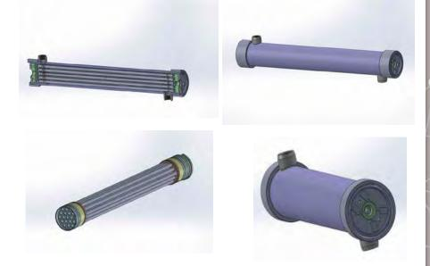
Figure 4: Potted module cross-section (left-most); new tube sheet module design (right).
