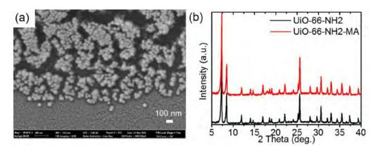
Figure 2: (a) SEM image of UiO-66-NH<sub>2</sub> nanoparticles; (b) XRD patterns of nanoparticles before and after the functionalization.
