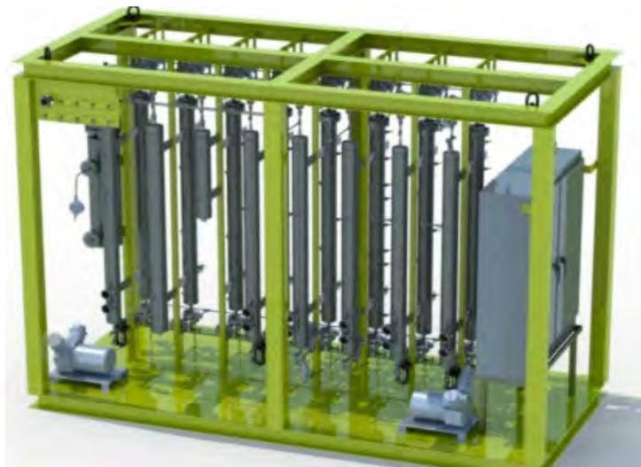
Figure 7: Eight-column integrated WGS and CO<sub>2</sub> capture unit.
