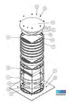
Figure 3: Detailed drawing of a membrane module stack containing eight membrane modules.
