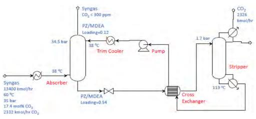
Figure 6: Configuration and operating conditions of the aMDEA process.
