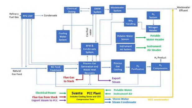
Figure 2: Flowsheet/block flow diagram of process.
