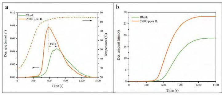
Figure 1: Catalytic effect of IL on CO<sub>2</sub> absorption and desorption. (a) Effect of CO<sub>2</sub> desorption rate with and without catalyst; (b) effect of catalyst on the quantities of desorbed CO<sub>2</sub>.
