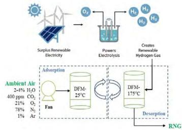
Figure 1: Block flow diagram for the overall DAC-DFM process using renewable H<sub>2</sub>.
