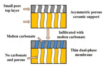
Figure 2: Physical structure of CCDP membrane.
