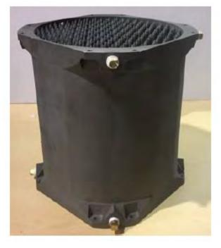
Figure 3: 3D-printed columns in plastic and metal.
