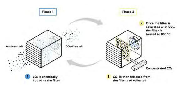
Figure 1: Schematic representation of Climeworks' adsorption and temperature-vacuum swing desorption processes for DAC.
