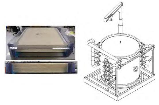
Figure 2: MTR CO<sub>2</sub> pre-concentrating membrane, internals on left and housing on right.
