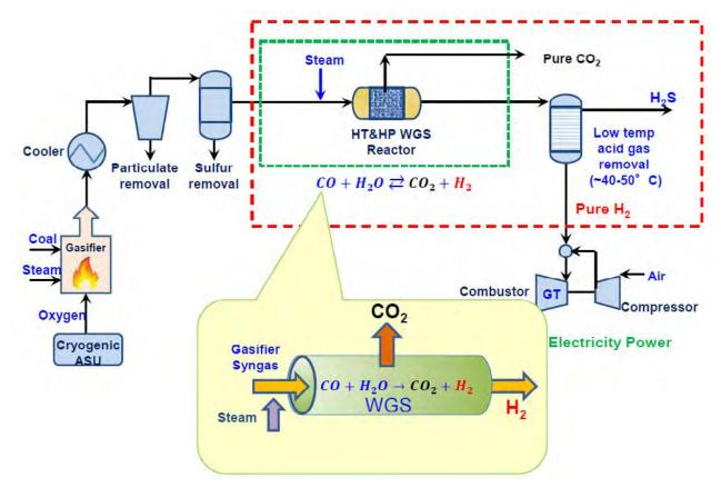
Figure 1: CCDP membrane reactor for WGS reaction and CO<sub>2</sub> capture in context of coal gasification plant cycle.
