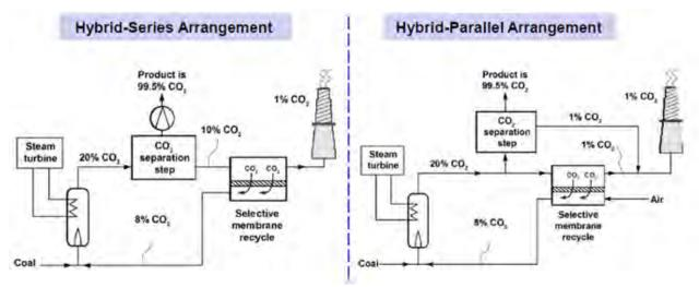
Figure 9: Two hybrid configurations for membrane-absorption CO<sub>2</sub> capture process.
