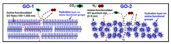
Figure 2: Membrane nanostructures of GO-1 and GO-2 membranes and proposed CO<sub>2</sub> separation mechanisms.
