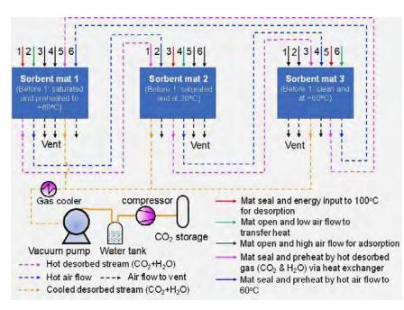
Figure 5: Proposed process flow for DAC.
