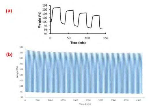
Figure 2: Degradation performance (@ 25°C, 400 ppm CO<sub>2</sub> in dry air) of (a) conventional aminopolymer/silica and (b) modified aminopolymer/silica.
