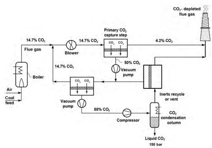
Figure 1: Simplified block diagram of the MTR large pilot CO<sub>2</sub> capture plant to be built.
