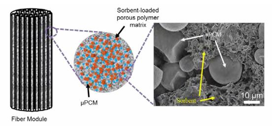
Figure 2: Phase-change material in hollow fiber sorbents.
