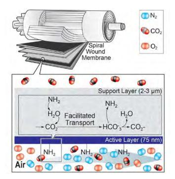
Figure 3: Schematic of facilitated transport mechanism for CO<sub>2</sub> separation from ambient air.
