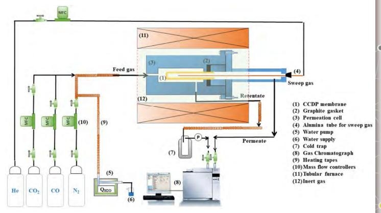
Figure 7: Laboratory-scale apparatus for CCDP membrane CO<sub>2</sub> permeation studies.
