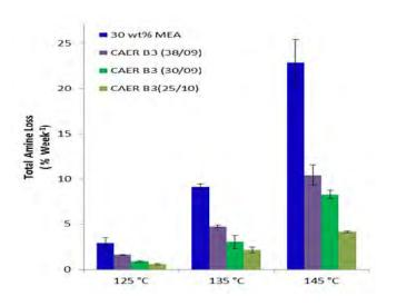
Figure 12: Rate of amine loss as total percent amine under stripper conditions of 30 wt% MEA (blue) and various combinations of CAER-B3.
