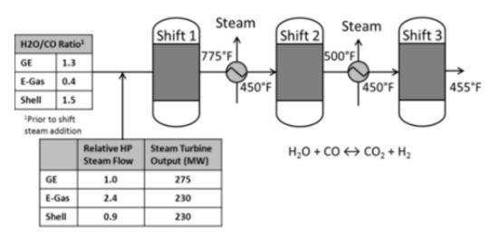
Figure 1: Three-stage, conventional WGS unit.
