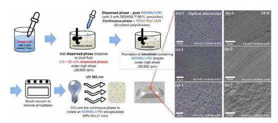
Figure 2: Synthesis of SIPs with NOHMs-I-PEI. (a) Optical microscope images of SIPs and (b) SEM images of the cross-section area of crosslinked SIPs film with different NOHMs loading: 9.8, 29.4, and 49.0 wt%. (Rim, G. et al. Advanced Functional Materials, 2021, 31(21), 2010047)
