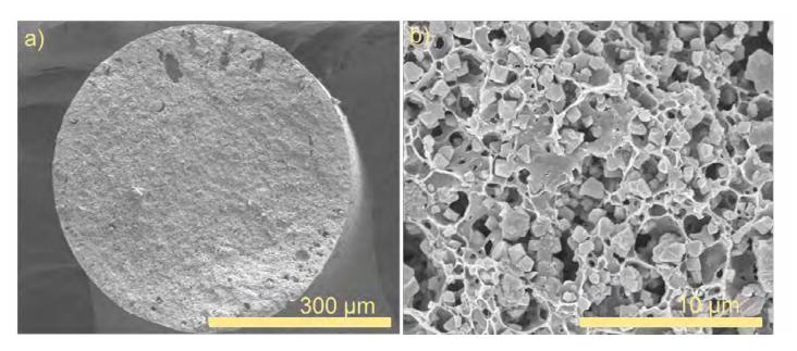
Figure 1: MIL-101(Cr)/cellulose acetate fiber sorbents: ~50 wt% MIL-101(Cr); (a) low magnification fiber, (b) zoomed in sub-structure.
