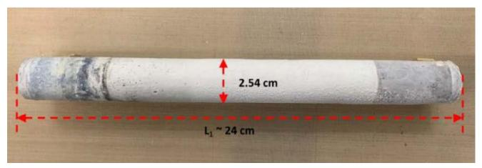
Figure 3: Post-heat-treated catalytic tube substrate.
