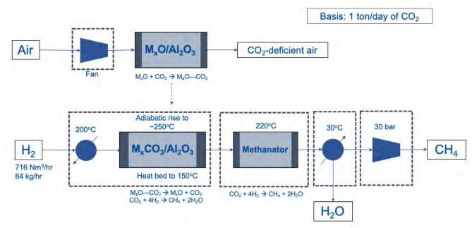
Figure 2: DAC-DFM with CO<sub>2</sub> capture at ambient conditions (25°C).
