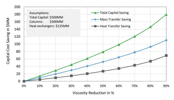
Figure 2: Impact of solvent viscosity reduction on the capital cost saving.
