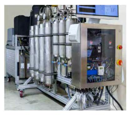
Figure 2:  $CO_2$  compression, storage, and upgrading skid.
