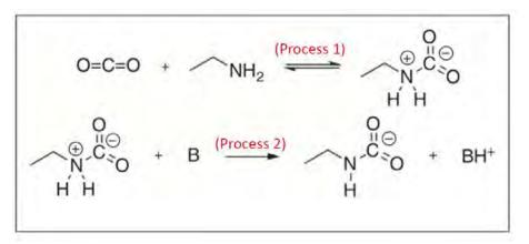
Figure 3: Mechanism of CO<sub>2</sub> capture involving (1) interaction between CO<sub>2</sub> and an amine followed by (2) deprotonation of resulting zwitterion in presence of a base.
