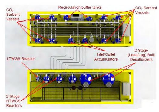
Figure 3: Overhead view of carbon capture skid.
