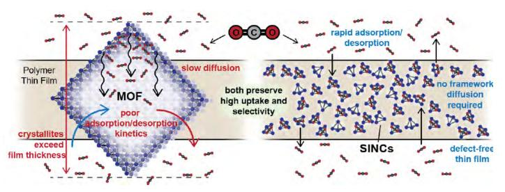
Figure 4: SINC sorbents preserve the high uptake and selectivity of MOFs for DAC while improving upon processability and the kinetics of capture and release of CO<sub>2</sub>.
