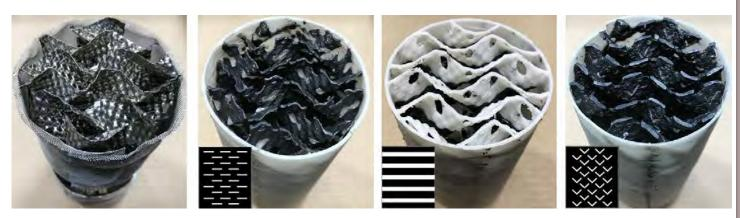
Figure 3: 250Y-type packing comparison with different dynamic design patterns (left to right) SS, DP-1, DP-2, DP-3.
