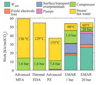
Figure 2: Comparison of capture work of thermal amine systems and EMAR systems.
