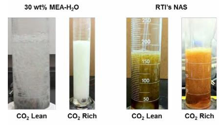
Figure 1: Comparison of foaming in aqueous and RTI's water-lean solvents.
