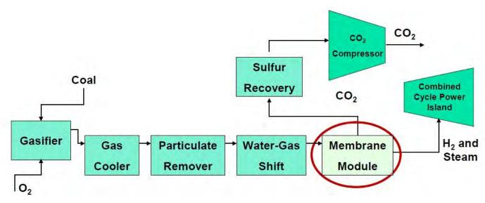
Figure 7: Flowsheet/block flow diagram showing PBI membrane module integration in the IGCC plant process.
