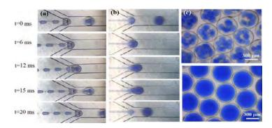
Figure 1: Encapsulated CO<sub>2</sub> capture solvent (NOHMs) produced using a microfluidic device.
