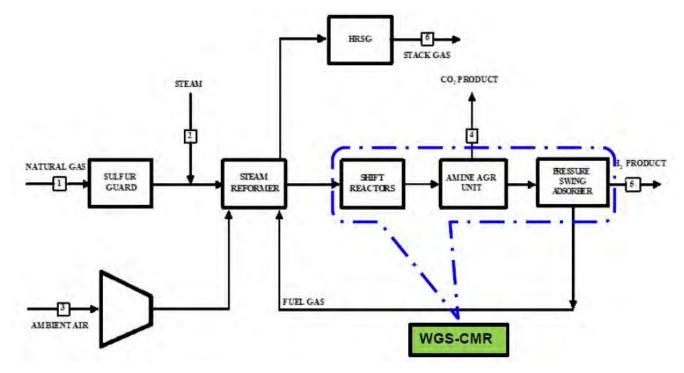
Figure 1: WGS-CMR (in green shadow) replacing two-stage shift, amine CO<sub>2</sub> capture, and PSA systems (in blue envelope) in natural gas steam reforming H<sub>2</sub> production process.
