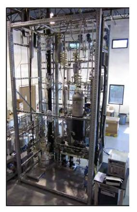
Figure 1: ION's lab-pilot (0.001 MWe) CO2 capture test unit.
