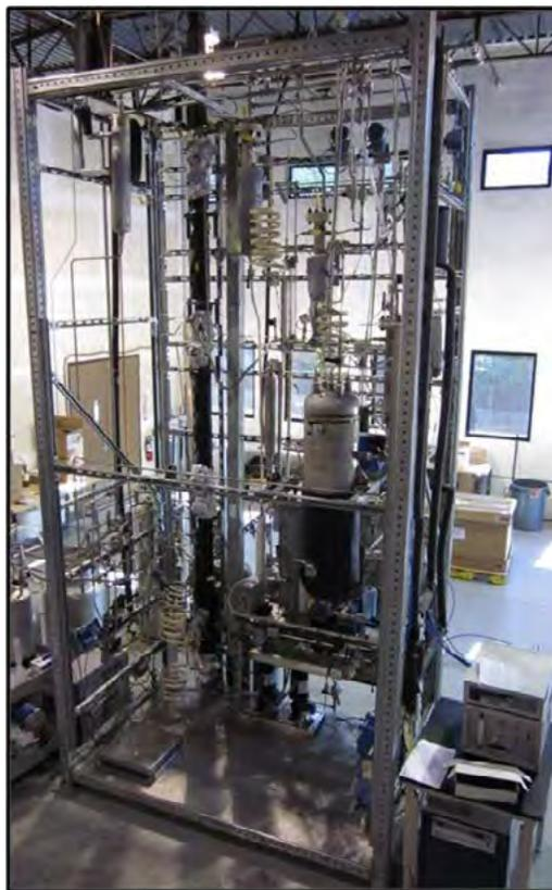
Figure 1: ION's lab-pilot (0.001 MWe) CO<sub>2</sub> capture test unit.
