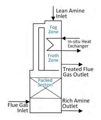
Figure 1: Schematic of University of Kentucky's compact absorber.
