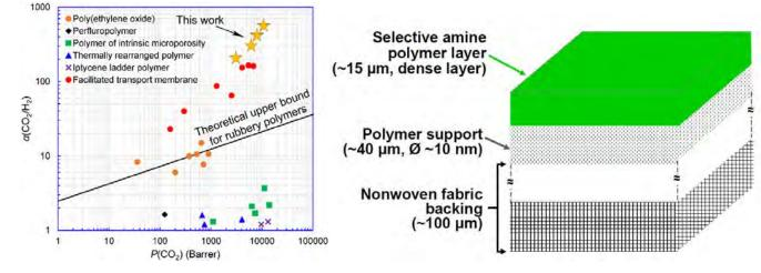
Figure 1: Typical performance of polymer membranes for CO<sub>2</sub>/H<sub>2</sub> separations.
