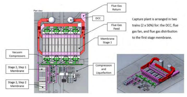
Figure 3: Final proposed membrane process equipment and layout.
