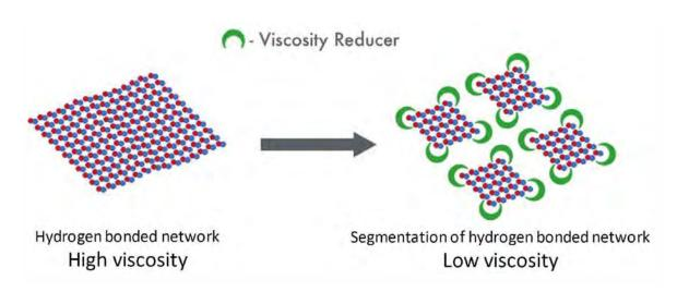
Figure 1: Illustration of fully HB network (left) and the breakage of the HB network by addition of HB acceptors (right).
