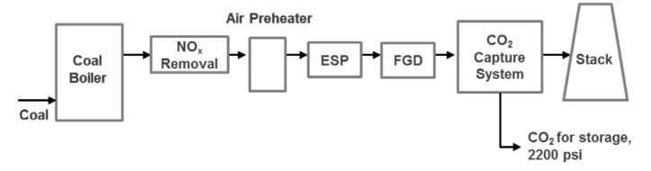
Figure 1: Schematic of TDA's CO<sub>2</sub> capture system.
