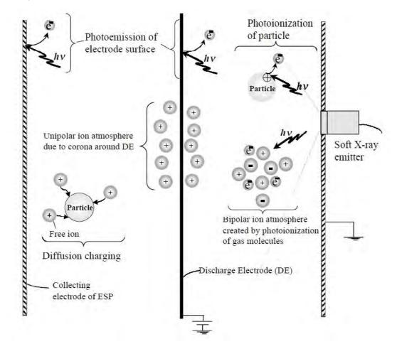
Figure 3: Conceptual flow diagram of the advanced ESP system developed by WUSTL.
