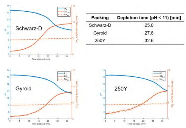
Figure 9: Relative comparisons of Schwarz-D, Gyroid, and 250Y structures. The Schwarz-D structure was found to be the best performing of the geometries.
