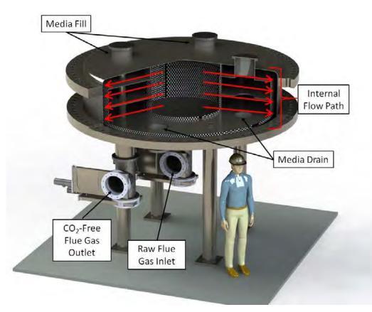
Figure 2: TDA Research's modular radial outflow reactor concept.
