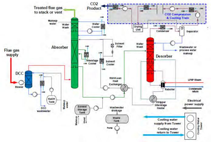
Figure 1: Linde-BASF carbon capture technology.
