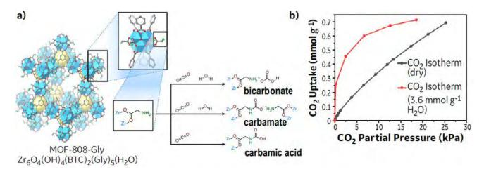
Figure 2: MOF-808-Gly benchmark MOF: (a) molecular structure and CO<sub>2</sub> adsorption mechanisms and (b) dry and humid CO<sub>2</sub> isotherms.
