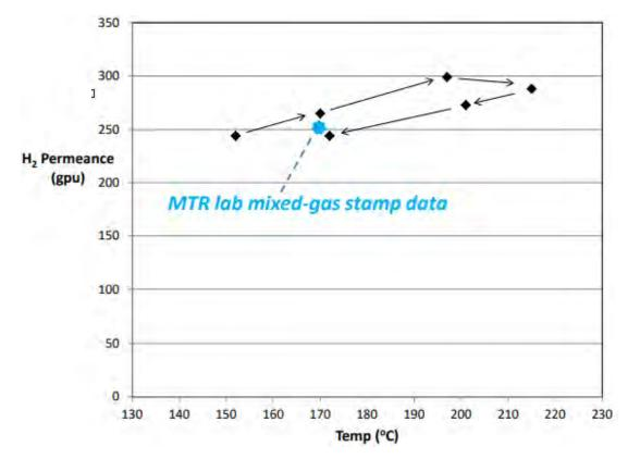
Figure 7: Influence of temperature on H<sub>2</sub> permeance during EERC field test of the Gen-2 Proteus module.
