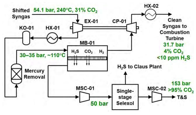
Figure 4: Process integration of membrane separation unit.
