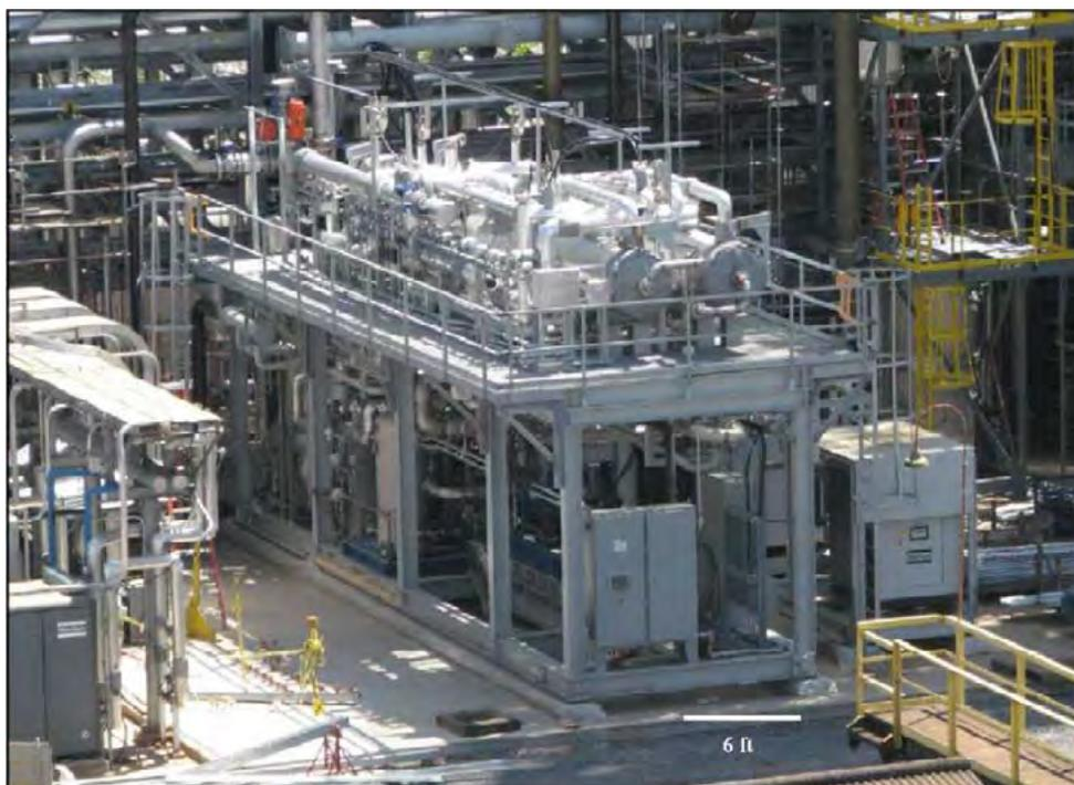
Figure 5: 20-TPD small pilot system installed at NCCC.
