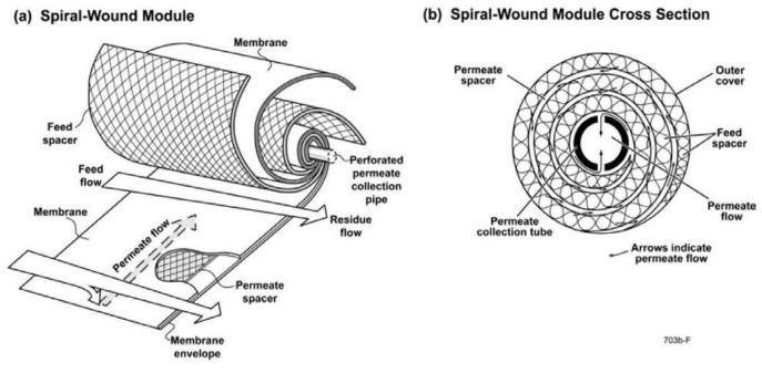
Figure 6: Schematic diagram of a spiral-wound membrane module.
