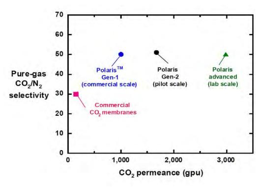
Figure 1: A CO<sub>2</sub>/N<sub>2</sub> trade-off plot showing data for several generations of MTR Polaris, compared with the properties of the standard commercial natural gas membrane. Data are pure-gas values at room temperature.
