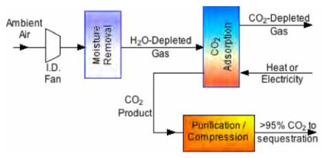
Figure 1: Process schematic for InnoSepra process.
