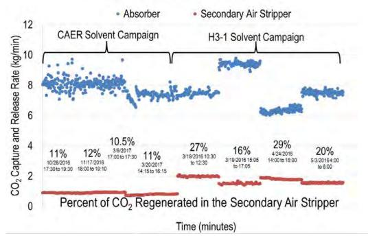
Figure 4: UK CAER secondary air stripper CO<sub>2</sub> regeneration.
