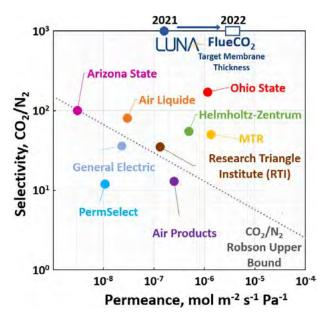
Figure 3: In a Robeson plot comparison, the Luna team's membrane (star) outperforms other CO<sub>2</sub> separation membrane technologies funded by the National Energy Technology Laboratory (NETL).
