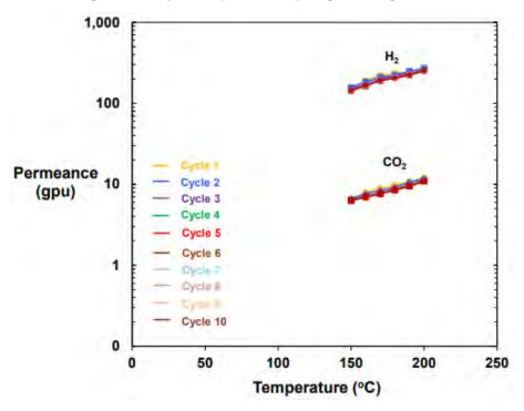
Figure 3: Gen-2 Proteus membrane temperature cycling results.
