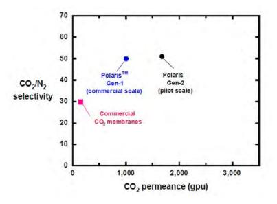
Figure 1: A CO<sub>2</sub>/N<sub>2</sub> trade-off plot showing data for two generations of MTR Polaris membrane. Data are pure-gas values at room temperature.
