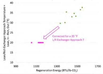
Figure 5: Effect of lean/rich heat exchanger approach temperature on solvent regeneration energy demand.
