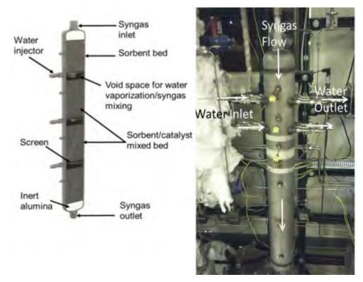
Figure 3: Bench-scale WGS and CO2 adsorption column.
