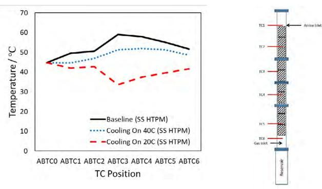
Figure 4: Heat transfer packing effect on absorber column temperature profile.
