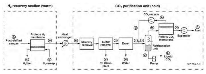
Figure 5: MTR dual-membrane process for H<sub>2</sub> recovery and CO<sub>2</sub> capture in IGCC power generation.
