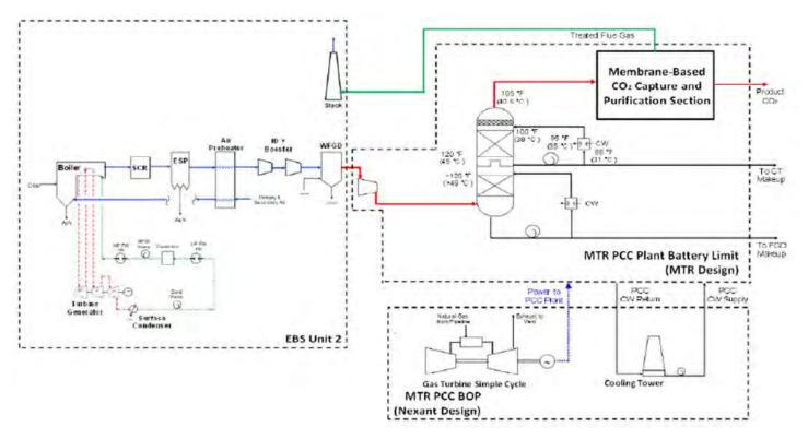
Figure 2: Proposed design for the East Bend unit.
