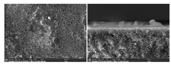
Figure 4: SEM images of the Si-ZNLM membrane: (left) surface and (right) cross-section.
