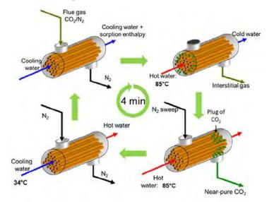
Figure 4: Rapid thermal swing adsorption cycle originally demonstrated for post-combustion CO<sub>2</sub> capture. Cycle times of 2.5–4.0 minutes have been demonstrated experimentally for 10% CO<sub>2</sub>.
