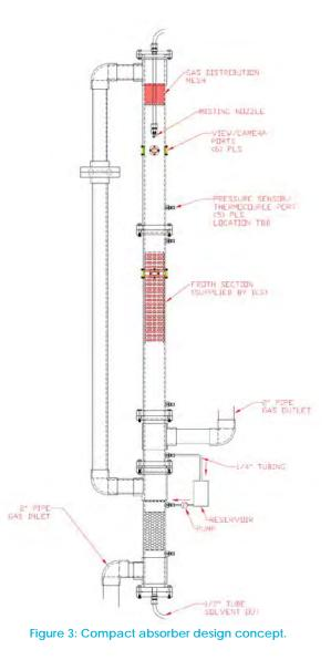
**Proposed Module Design** – The absorber is modular with a natural divide between the bottom packed section and the top fog and froth section.
