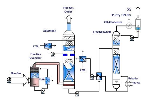
Figure 2: Carbon capture basic process flow diagram.
