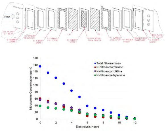
Figure 5: Flow-through e-cell schematic with CX electrodes (top) and nitrosamine destruction to below detection limit within 12 hours of electrolysis (bottom).
