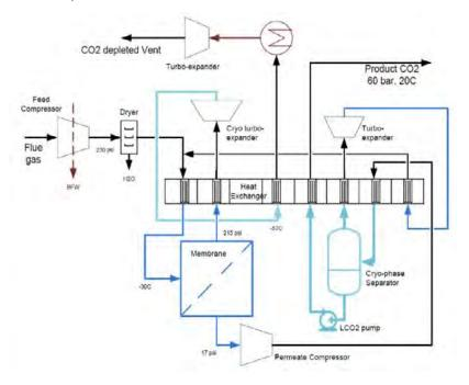
Figure 2: Schematic diagram of cold membrane process.
