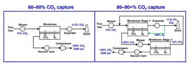
Figure 3: Flow diagrams of a one-stage membrane process to achieve 60–80% capture (left) and an innovative process to achieve >80% capture (right).
