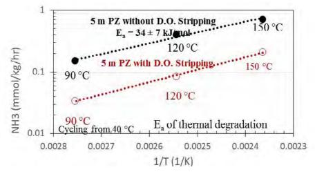
Figure 3: N<sub>2</sub> sparging reduces oxidation in high-temperature oxidation reactor (HTOR) by a factor 3.5–4.5. Cycling from 40°C with 0.1 mmol Fe<sup>+2</sup>/kg. At 40°C absorption/40°C stripping, the ammonia (NH<sub>3</sub>) production rate (0.025 mmol/kg-hr) would be negligible. (Nielsen, 2018)
