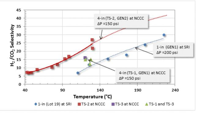
Figure 5: Comparison of measured H<sub>2</sub>/CO<sub>2</sub> selectivity for Gen-1 and Gen-2 PBI modules.
