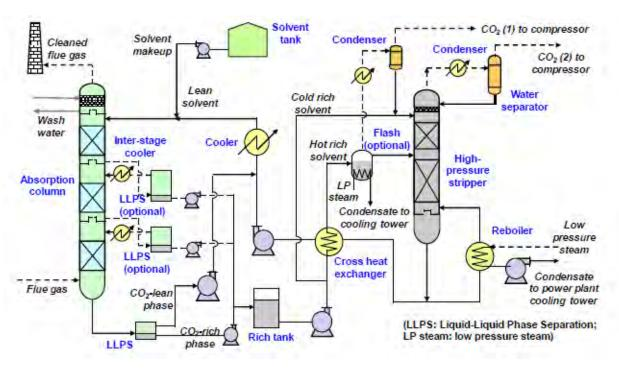
Figure 2: Schematic diagram of the BiCAP with multiple stages of LLPS.
