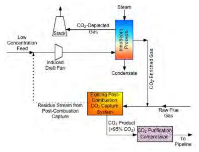
Figure 1: InnoSepra capture process.
