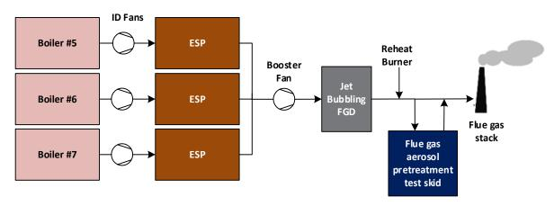
Figure 5: Abbott Power Plant layout and connection to flue gas aerosol pretreatment test skid.
