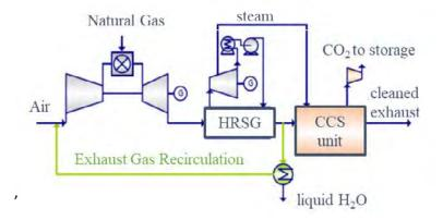
Figure 2: Exhaust gas recirculation.
