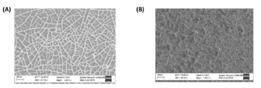
Figure 4: Variation in metal oxide coating morphology.
