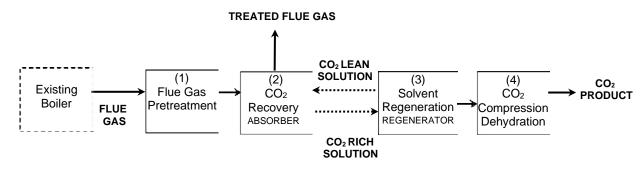
Figure 1: Block flow diagram of the CO<sub>2</sub> recovery plant.
