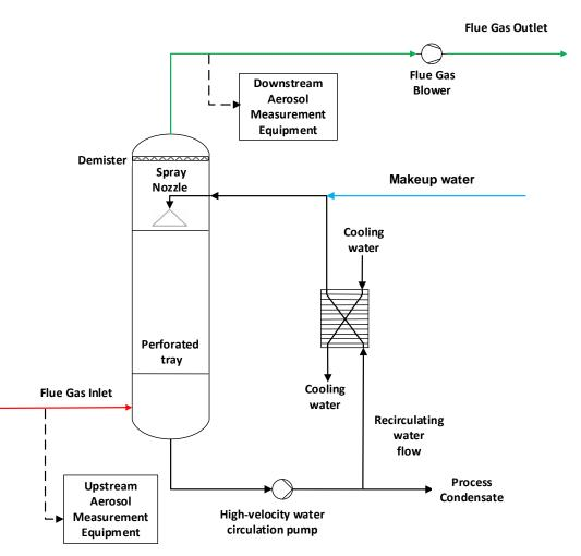
Figure 2: Process flow diagram of high-velocity water spray-based aerosol pretreatment system.
