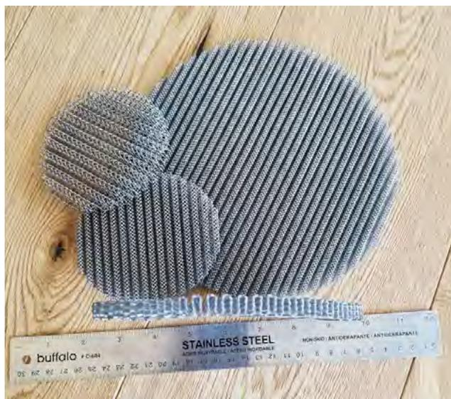
Figure 2: Froth-generating and -propagating screens.
