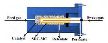
Figure 10: WGS reaction in membrane reactor with Co-Mo-Mg(AlO<sub>2</sub>)<sub>2</sub>-based shift catalyst.
