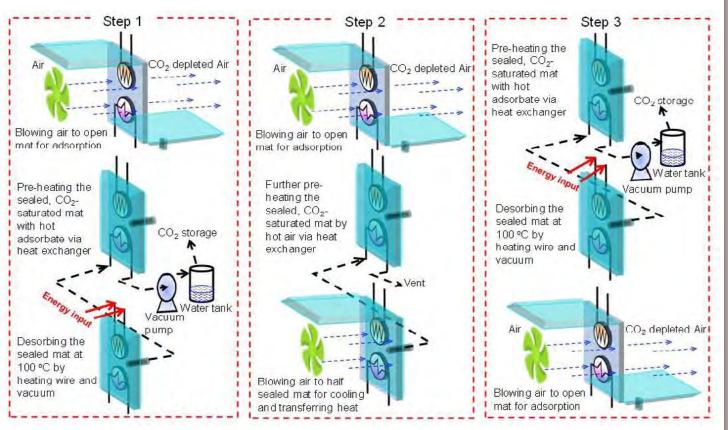
Figure 2: Diagram of the process for DAC.
