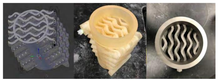
Figure 3: 3D-printed packing.
