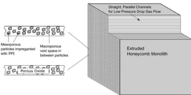
Figure 1: Monolith system used in Global Thermostat process.
