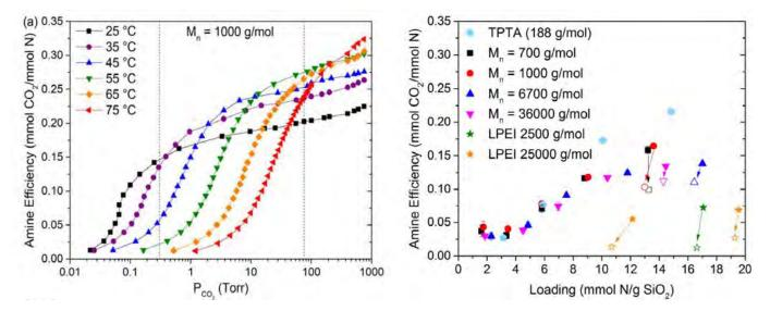
Figure 3. Left: Isotherms at varied temperatures for PPI/SBA-15 sorbents. Right: Amine efficiency versus amine loading for I-PPI versus PEI (closed shapes), 400 ppm CO<sub>2</sub> at 35°C, showing loss after treatment in oxidative environment (open shapes), 21%O<sub>2</sub>/N<sub>2</sub>, 110°C for 24 hours.
