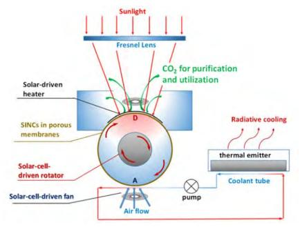
Figure 1: Integrated electricity-free radiative cooling, membrane adsorption, solar heating and desorption, and CO<sub>2</sub> product for further purification and utilization.
