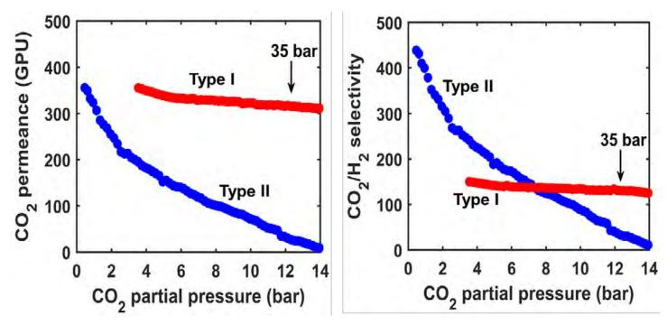
Figure 6. CO<sub>2</sub> permeances and CO<sub>2</sub>/H<sub>2</sub> selectivities of membranes incorporating the Type I and Type II mobile carriers in simulated syngas at 107°C and 35 bar.
