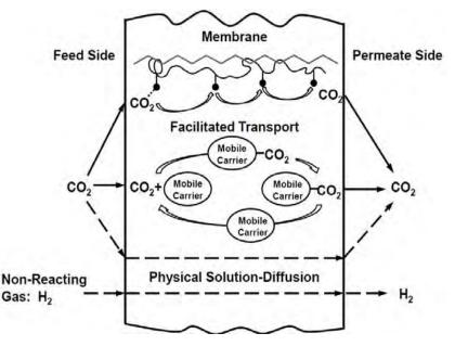
Figure 3: Mechanism of facilitated transport.
