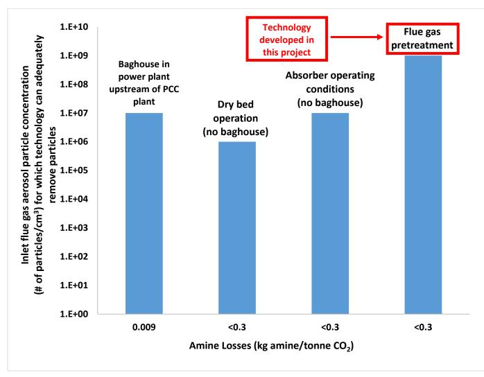
Figure 1: Flue gas aerosol particle number concentration ranges for which aerosol mitigation technologies are applicable and sufficient.
