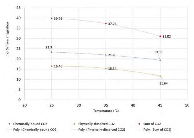
Figure 2: VLE for 50:50 DEEEA: EEMPA for  $CO_2$ : H<sub>2</sub> (1:1) gas mixture at 35 bar.
