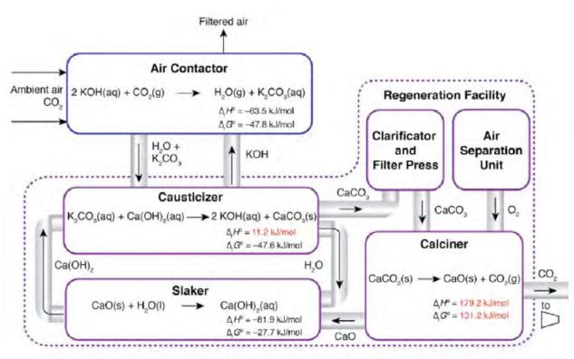
Figure 1: Solvent-based direct air capture system.
