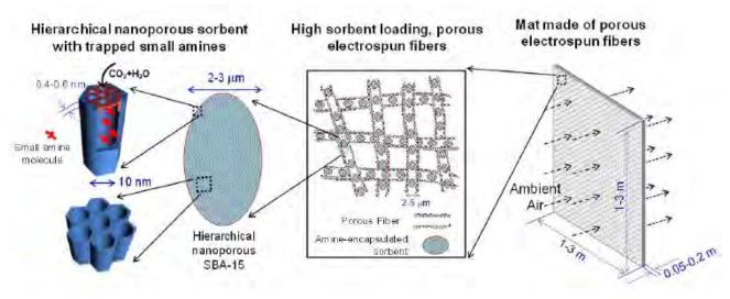
Figure 1: Diagram of the transformational adsorbent for direct capture of  $CO_2$  from air.
