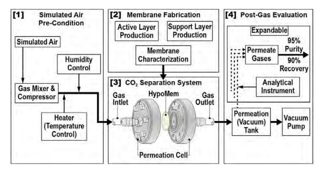
Figure 4: An illustration of the HypoMem CO<sub>2</sub> separation system.
