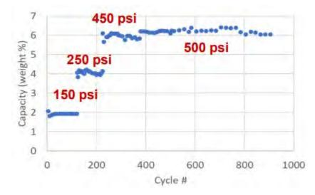
Figure 5: TDA capture sorbent CO<sub>2</sub> capacity.
