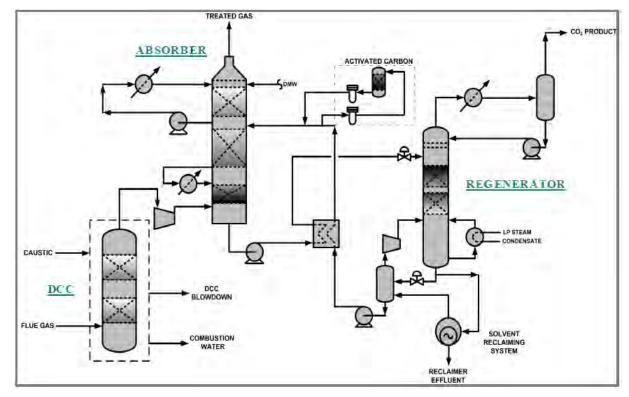
Figure 1: Schematic of Fluor's EFG+ CO<sub>2</sub> capture technology.
