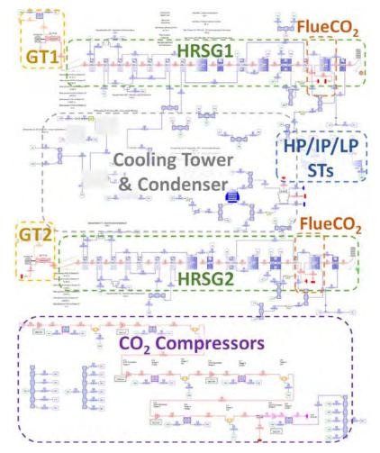
Figure 6: Thermoflex model of FlueCO<sub>2</sub> NGCC.
