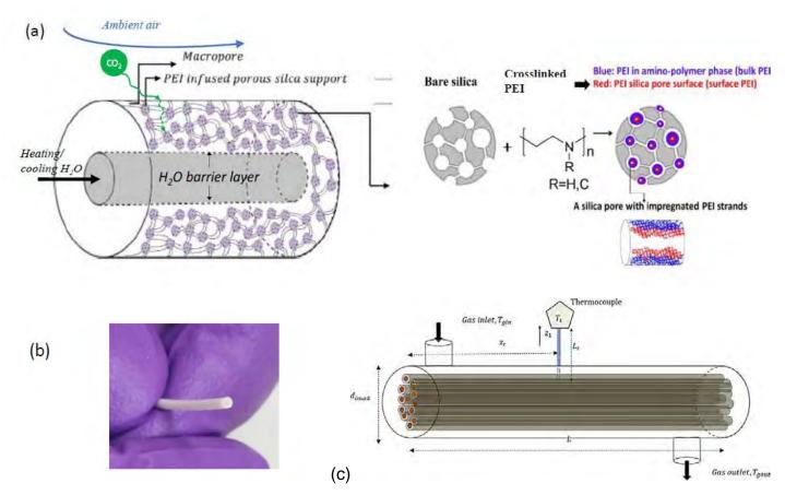
Figure 1: (a) General structure of the BIAS particles and envisioned test setup/CO<sub>2</sub> capture scheme for the hollow-CHEFS, (b) hollow-CHEFS photo image developed at NETL, and (c) schematic of a hollow-CHEFS membrane module<sup>1</sup>.
