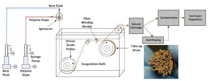
Figure 6: LANL lab-scale continuous hollow fiber spinning system.
