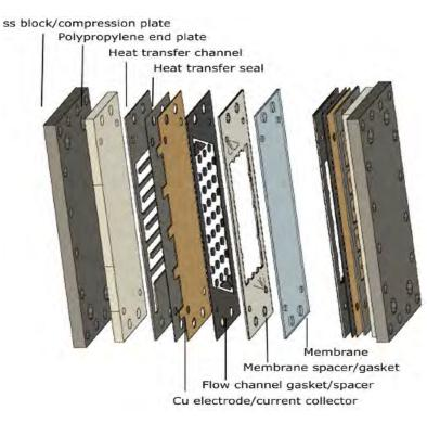
Figure 3: Electrochemical single-cell engineering.
