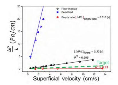
Figure 3: Pressure drop comparison and targets. Target pressure drop for this work is 250 Pa at 3 m/s air speed and is shown by the green line.
