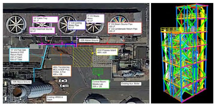
Figure 1: (Left) Overhead view of LMEC with 1,600-ft<sup>2</sup> (150 m<sup>2</sup>) pilot site and required tie-ins identified. (Right) Image of the 3D model of the modular system.
