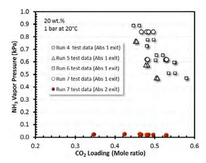
Figure 4: Measured NH<sub>3</sub> vapor pressure at various CO<sub>2</sub> loadings for tests conducted with a single absorber (Runs 4, 5, and 6) and for the test conducted with the dual absorber (Run 7).
