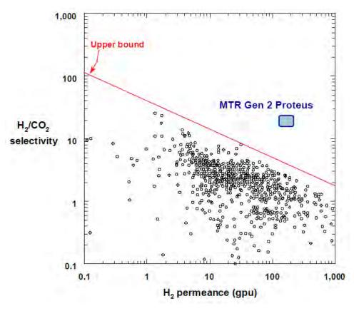
Figure 2: Robeson plot with Gen-2 Proteus membrane performance.
