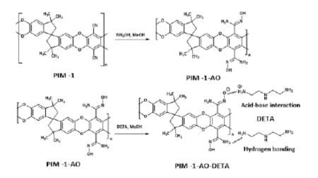
Figure 2: Reaction scheme and preparation of PIM-1-AO-DETA sorbent.
