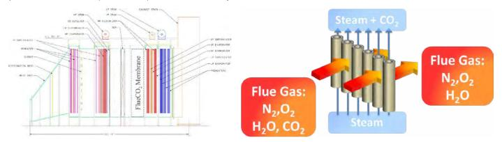
Figure 1: Luna's dual-phase membrane technology introduces a unique ability to implement carbon capture technologies into power plant HRSGs (150–500°C).
