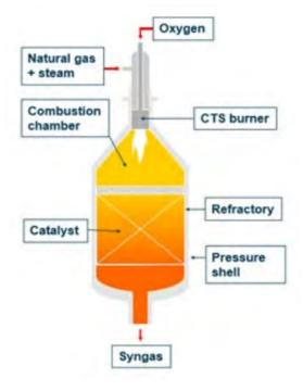
Figure 2: SynCOR™ autothermal reformer.
