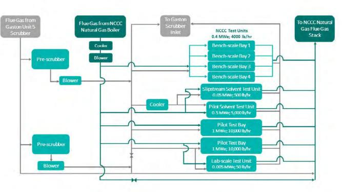
Figure 1: Diagram of post-combustion test facilities at the National Carbon Capture Center.
