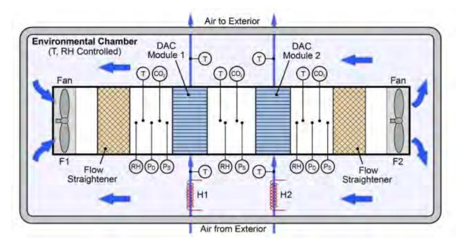
Figure 1: Test chamber for long-term testing of contactor modules.
