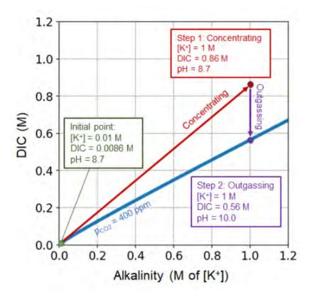
Figure 1. The ACS cycle (concentrating and outgassing steps).
