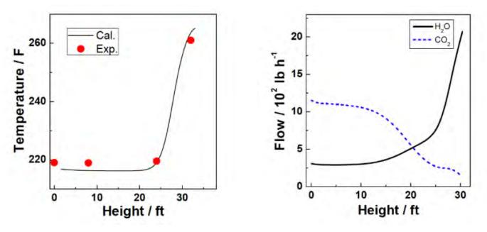
Figure 7: Temperatures and mass fluxes in solvent stripper.
