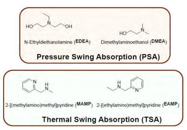
Figure 1: Certain non-proprietary amine solvents tested for CO<sub>2</sub> capture.
