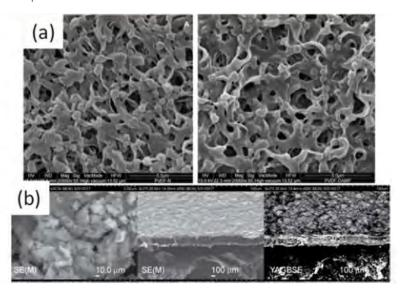
Figure 3: (a) Typical Scanning electron microscopy (SEM) photo of the surface of a porous PVDF membrane, (b) SEM of the hybrid PVDF and example SINCs (copper-MOF).
