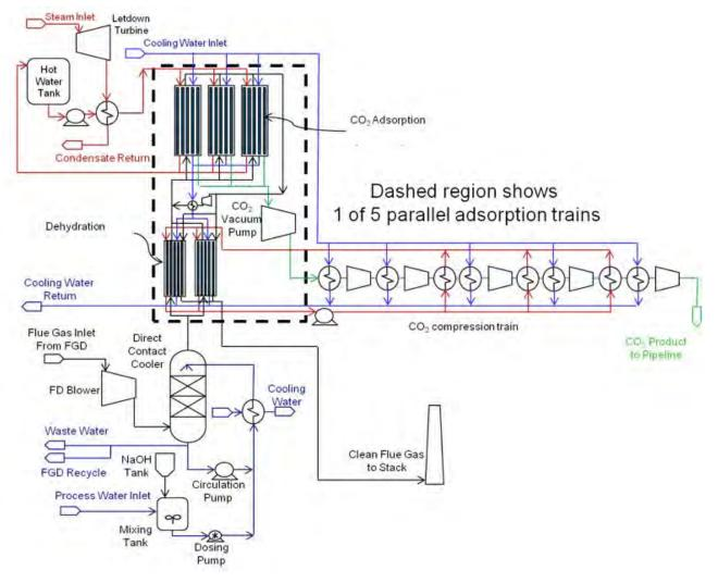
Figure 3: Commercial process configuration.
