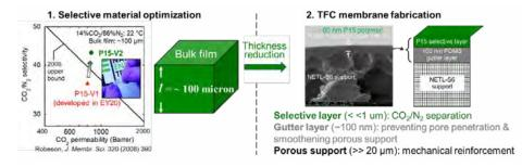
Figure 3: Selective layer material optimization and TFC development.
