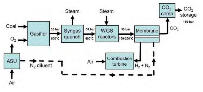
Figure 4: Overall process design for the pre-combustion capture membrane system.
