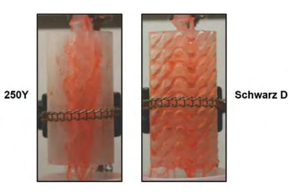
Figure 5: Fluid flow through conventional packing geometry (left) and TPMS packing geometry (right).
