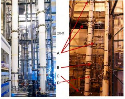
A: Rich solution inlet locations B: Discharge locations for high NH<sub>3</sub>/K solution C: Discharge locations for low NH<sub>3</sub>/K solution D: Heat exchangers (Cold rich↔ Hot lean)
