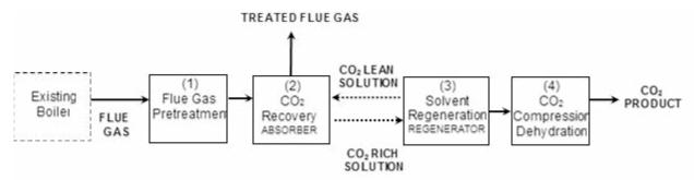
Figure 1: Block flow diagram of the CO<sub>2</sub> recovery plant.
