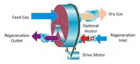
Figure 2. Rotating wheel dryer for feed dehumidification.
