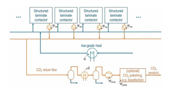
**Proposed Module Design** – The full-scale plant design will integrate Climeworks' modular DAC "collectors" with Svante's modular structured adsorbent beds. This is a fixed-bed, structured sorbent (laminates) approach. The flowrates in Table 1 above are for individual modules for the test plant being built in California for this project.
