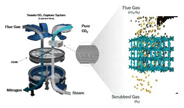
Figure 1: VeloxoTherm<sup>™</sup> Rotary Adsorption Machine.
