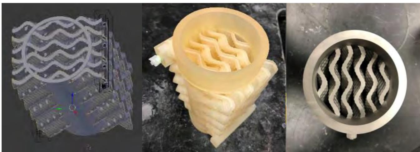
Figure 3: 3D-printed packing.
