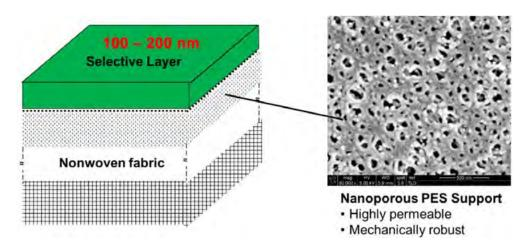
Figure 1: Schematic of thin-film composite membrane consisting of an amine-containing cover layer on a nanoporous PES support.
