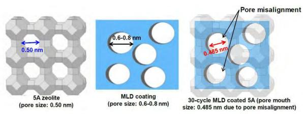
Figure 1: Schematic of pore misalignment for fine-tuning pore mouth size of sorbents.
