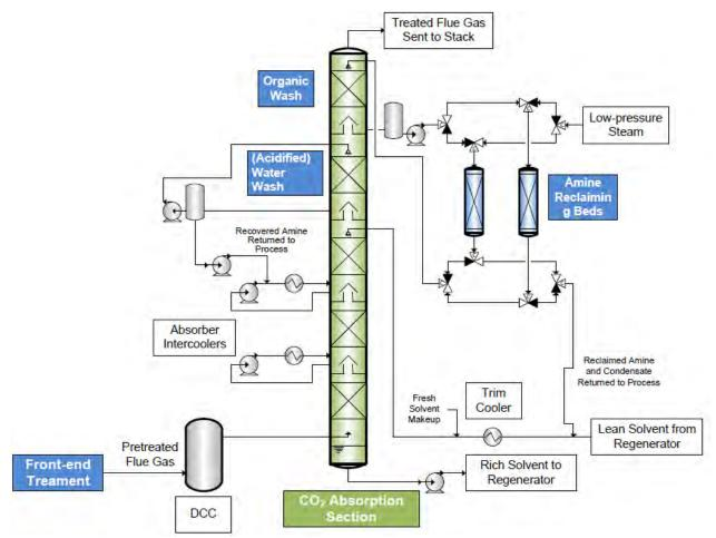
Figure 1: Potential ECTs for WLS systems to be incorporated at a CO<sub>2</sub> capture plant.
