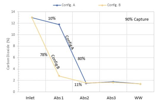
Figure 7: CO<sub>2</sub> capture efficiency profiles for configurations A and B (total of 90% capture in both cases).
