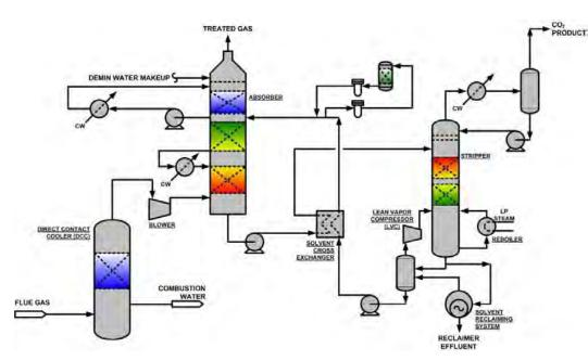
Figure 1: Simplified schematic of Fluor Corporation's Econamine FG Plus™ CO₂ capture process.
