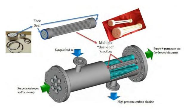
Figure 2: Permeate purgeable multiple bundle housing and seals.
