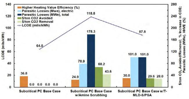
Figure 5: Comparison of the cost of CO<sub>2</sub> capture between DOE/NETL Base Case 9 (subcritical PC plant without CO<sub>2</sub> capture), Base Case 10 (subcritical PC plant with amine scrubbing), and the MLD-coated sorbent/PSA process.
