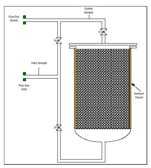
Figure 4: Process flow diagram of the InnoSepra sorbent-based filter technology.
