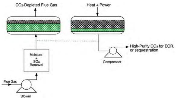
Figure 1: InnoSepra capture process schematic.
