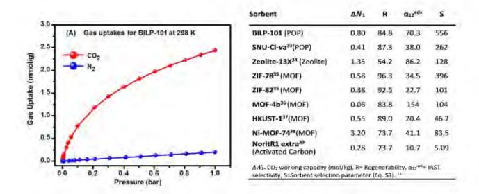
Figure 1:  $CO_2$  and  $N_2$  adsorption isotherm of the BILP sorbent and the list of top-performing sorbents for flue gas ( $CO_2/N_2$ :10/90) separation using vacuum swing adsorption at 298K,  $P_{ads}$ =1 bar, and  $P_{des}$ =0.1 bar.
