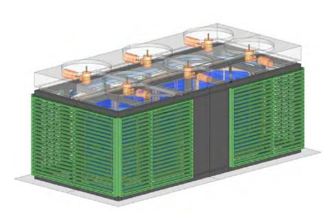
Figure 1: 3D rendering of GT's DAC system, with nine stations for sorption and one station for harvest/regeneration (gray area in Figure).
