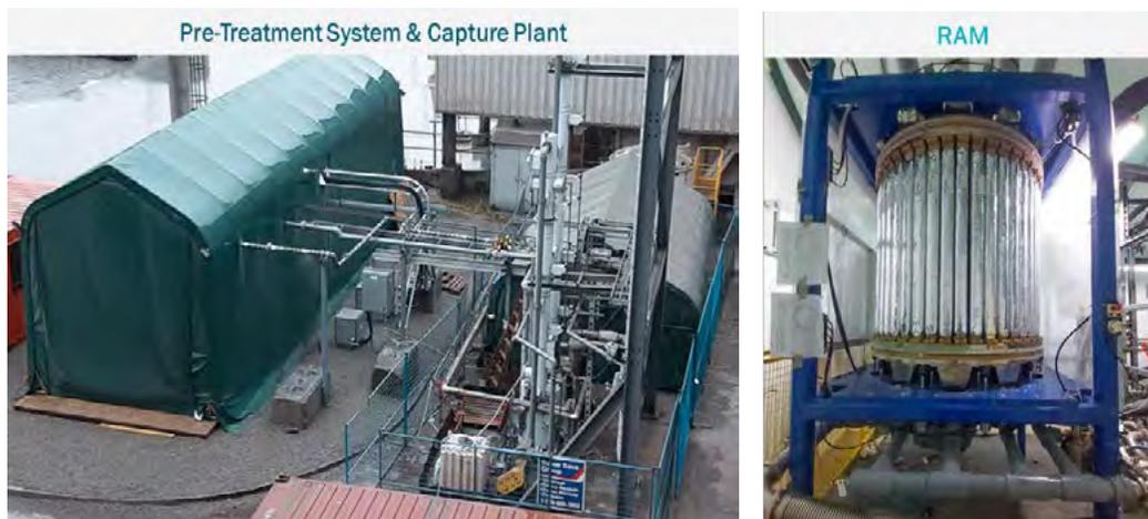
Figure 3: CO<sub>2</sub>MENT field Unit (1 TPD) at a Lafarge cement plant in Richmond BC showing the pre-treatment system and capture plant (left) and the RAM showing the beds (right).
