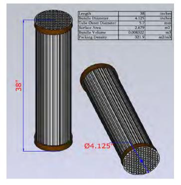
Figure 6: Dewatering membrane module design.
