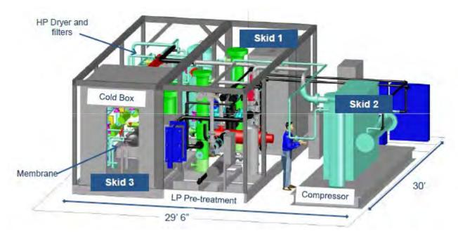
Figure 3: 0.3-MWe test unit at NCCC, Pilot Bay 3.
