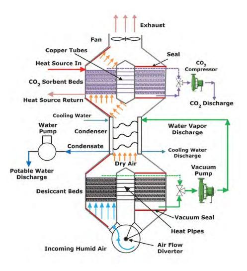
Figure 1: Schematic of HDAC concept.
