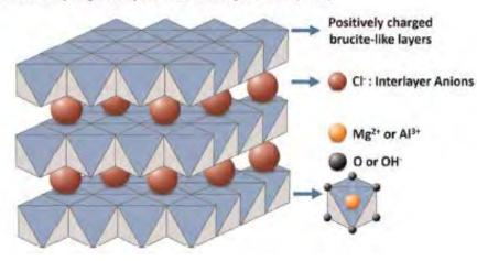
Anionic clay Mg/Al-layered double hydroxide (LDH)
