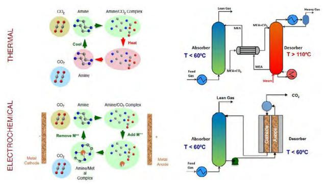
Figure 1: Electrochemically mediated versus thermal amine regeneration.
