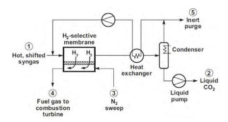
Figure 8: Membrane process integration in process cycle.
