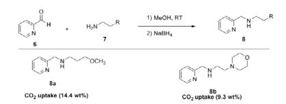
Figure 2: Synthetic methodology for the synthesis of third-generation aminopyridine derivatives.
