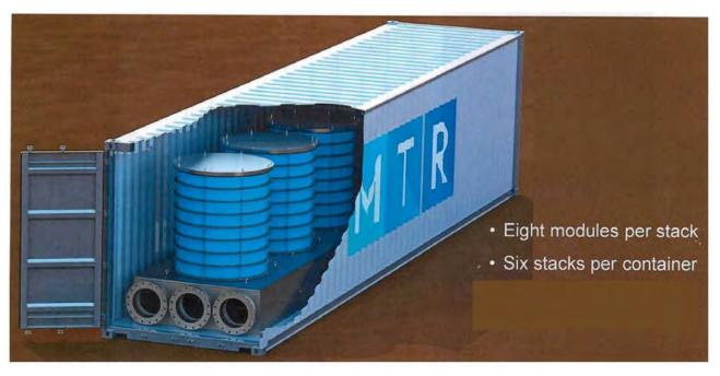
Figure 3: SolidWorks drawing showing the form of a containerized skid housing six membrane module stacks. Each stack is composed of eight modules.
