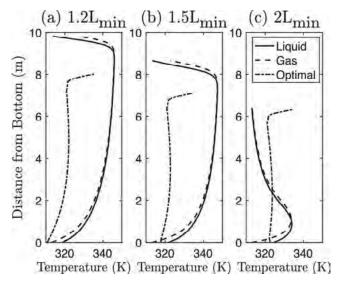
Figure 11: Optimal and adiabatic temperature profiles under conditions for (a) 1.2 L<sub>min</sub>, (b) 1.5 L<sub>min</sub>, and (c) 2 L<sub>min</sub>.
