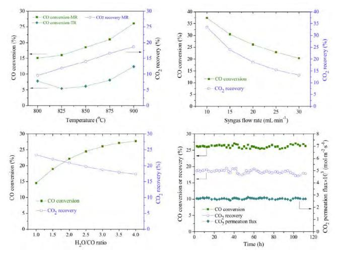
Figure 8: Measurements from tubular CCDP modules in high-temperature WGS testing (1 atm feed).
