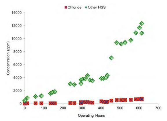
Figure 6: Accumulation of contaminants in solvent.
