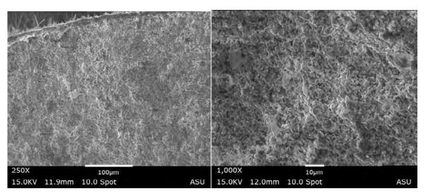
Figure 3: SEM images of CCDP membrane cross-section at 250x (left) and 1,000x (right).
