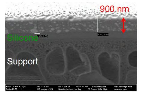
Figure 4: Cross-sectional scanning electron microscopy (SEM) of membranes.
