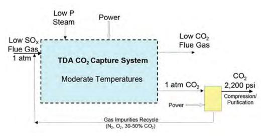
Figure 1: Block flow diagram of TDA's CO<sub>2</sub> capture system.
