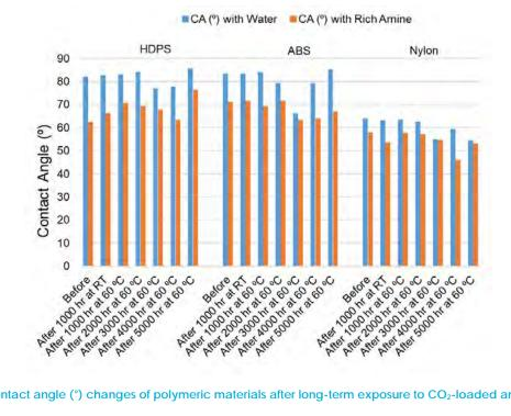
Figure 1: Contact angle (°) changes of polymeric materials after long-term exposure to CO<sub>2</sub>-loaded amine solvent.
