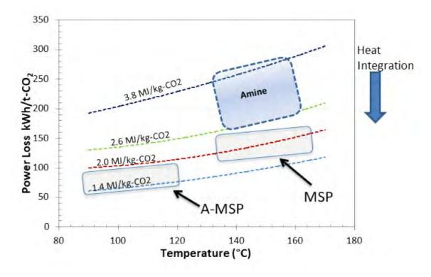
Figure 3: Power plant energy loss due to steam extraction.
