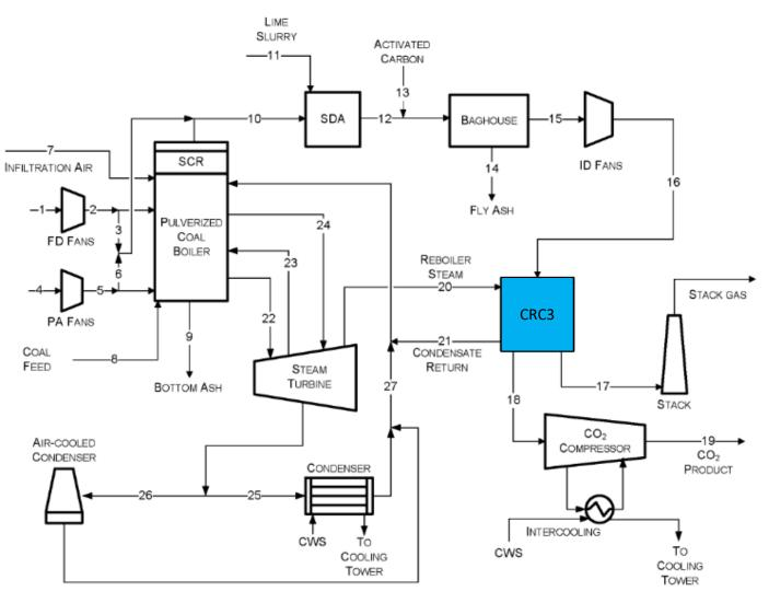
Figure 4: Process concept for the CRC3 system.
