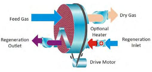
Figure 2: Rotating wheel dryer for feed dehumidification.
