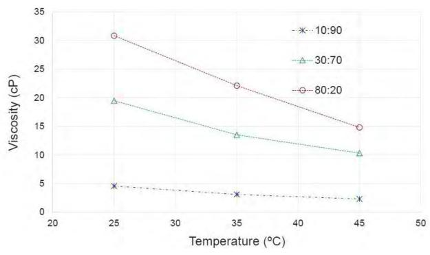
Figure 3: Viscosity versus temperature of DEEEA: EEMPA blends under 500 psi CO<sub>2</sub>.
