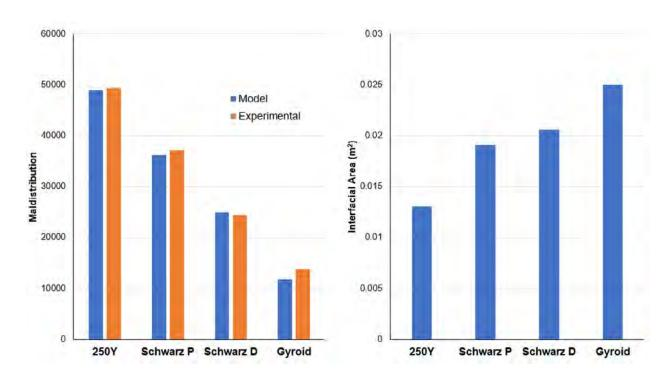
Figure 7: Liquid maldistribution and interfacial area of different geometries. TPMS structures all exhibit better liquid flow properties compared to conventional 250Y geometries.
