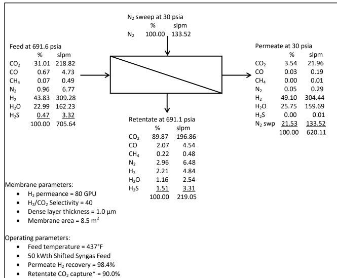
Retentate CO<sub>2</sub> dry basis purity = 96.88% after H<sub>2</sub>S removal and catalytic oxidation of CO, H<sub>2</sub> and CH<sub>4</sub>
