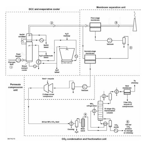
Figure 1: Preliminary design for full-scale membrane capture plant.
