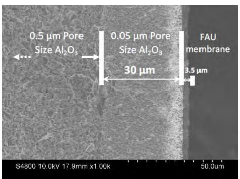
Figure 5: Dewatering membrane structure.
