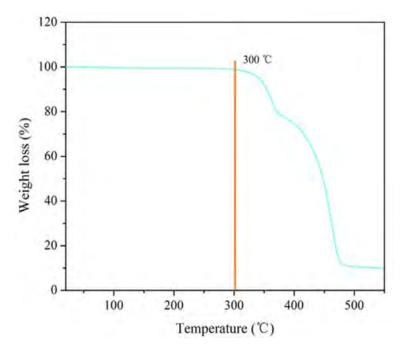
Figure 3. The TGA trace of (EMmim<sup>+</sup>)(NTF<sup>2-</sup>) at 10°C heating rate.
