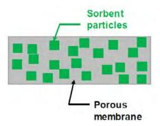
Figure 2: Flat-sheet membrane adsorbents with porosity 60–95% comprising CO<sub>2</sub>-philic SINCs and polymers.
