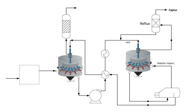
Figure 2: ROTA-CAP bench-scale test skid process flow diagram.
