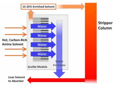
Figure 3: Solvent membrane dewatering for CO<sub>2</sub> enrichment.
