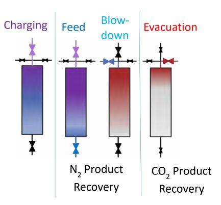
Figure 4: Pressure swing adsorption process.
