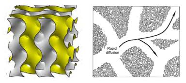
Figure 1: Design features focused on at LLNL: triply periodic minimal surface (left), hierarchical flow channels (right).
