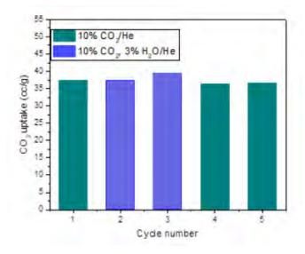
Figure 4: Preliminary CO<sub>2</sub> uptake performance of NETL's high-performance m-poly-1 tested in packed-bed reactor with gas breakthrough analysis under dry and humid conditions.
