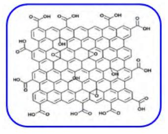
Figure 1: Chemical structural model of GO.
