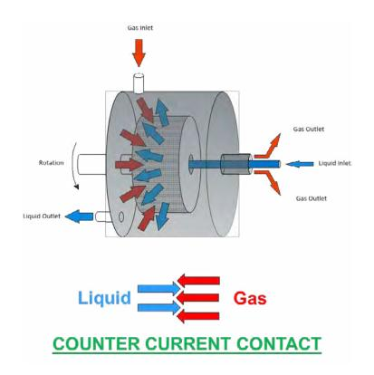
Figure 1: RPB gas-liquid contactor.
