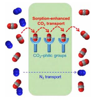
Figure 2: The highly branched amorphous polymers containing poly(1,3-dioxolane) (PDXL) in the branches interact favorably with  $CO_{2}$ , but not  $N_{2}$ , allowing for the design of solubility-selective membrane materials with superior performance for gas separations.
