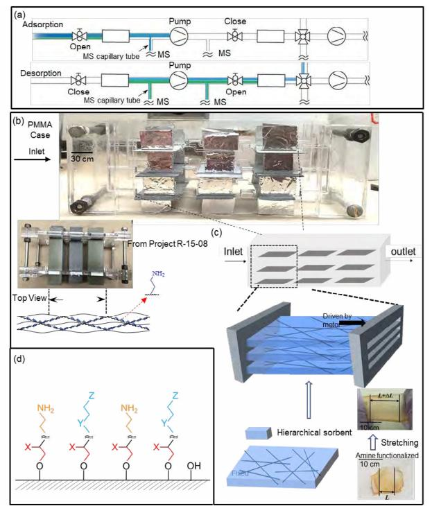
Figure 4. Vacuum swing adsorption for CO<sub>2</sub> capture from air (a) VSA scheme, (b) a VSA unit with sorbent plates in a plexiglass (i.e., PMMA) case, (c) the arrangement of sorbent plates in a parallel configuration, (d) the structure of amine sites for weakly adsorbed CO<sub>2</sub>. X, Y, and Z denote different types of functional groups.
