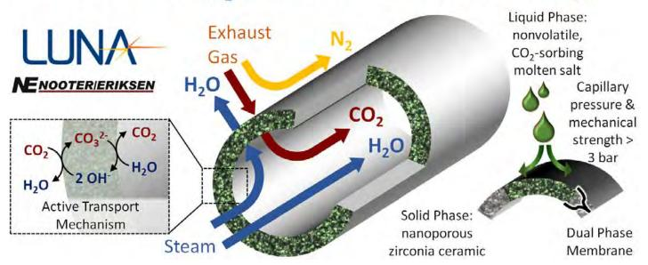
Figure 2: Luna Innovations dual-phase membrane technology for highly efficient and scalable CCS.
