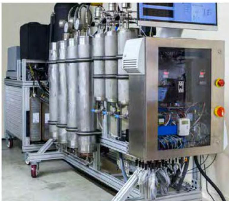
Figure 2: CO<sub>2</sub> compression, storage, and upgrading skid.
