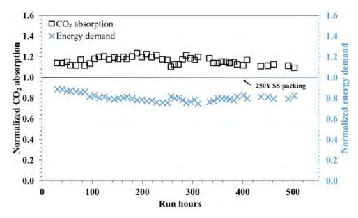
Figure 4: CO<sub>2</sub> absorption efficiency and energy demand during the 500-hour long-term testing.
