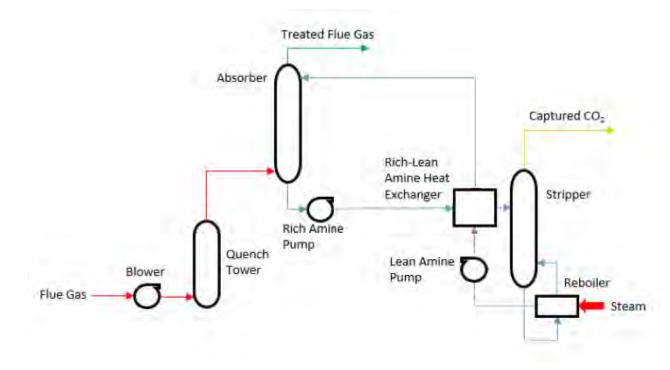
Figure 1: Generic simplified flowsheet for amine-based CO<sub>2</sub> capture from flue gas.
