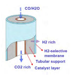
Figure 2: WGS-CMR tubular configuration.
