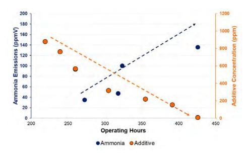
Figure 8: Ammonia emissions versus additive in the solvent.
