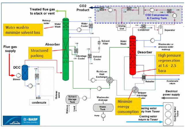
Figure 1: Process design with key features highlighted.
