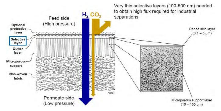
Figure 1: Proteus membrane multi-layer composite structure.
