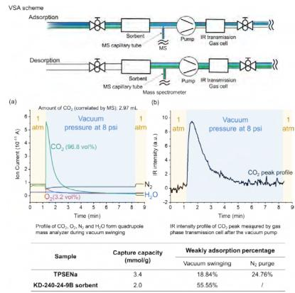
Figure 3. VSA Scheme—Adsorption by flowing a 0.04% CO<sub>2</sub> stream over a sorbent bend; desorption of weakly adsorbed species by vacuum. The concentration profiles of the effluent form adsorption bed under 8 psi vacuum determined by (a) MS before vacuum pump, (b) infrared gas cell after vacuum pump. (1 atm=14.7 psi)
