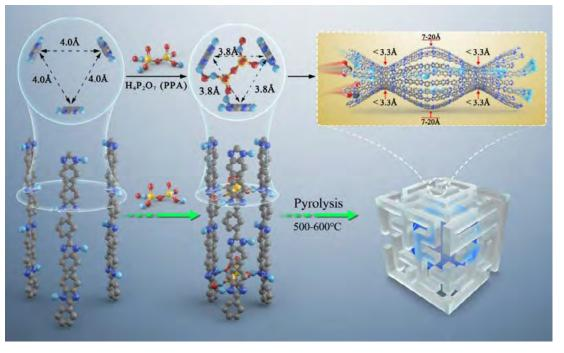
Figure 2: Steps to CMS membranes derived from PBI doped with polyprotic acids.
