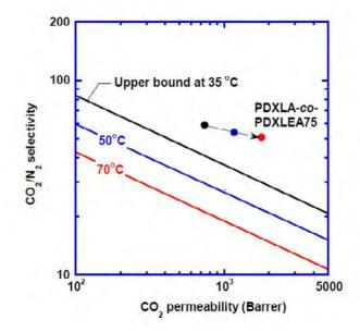
Figure 1: The "rubbery polymers": two macromonomers, poly(1,3-dioxolane) acrylate (PDXLA) and poly(1,3-dioxolane) ethyl ether acrylate (PDXLEA) are highly polar polymers that exhibit  $CO_2/N_2$  separation properties above the upper bound in the Robeson's plot.
