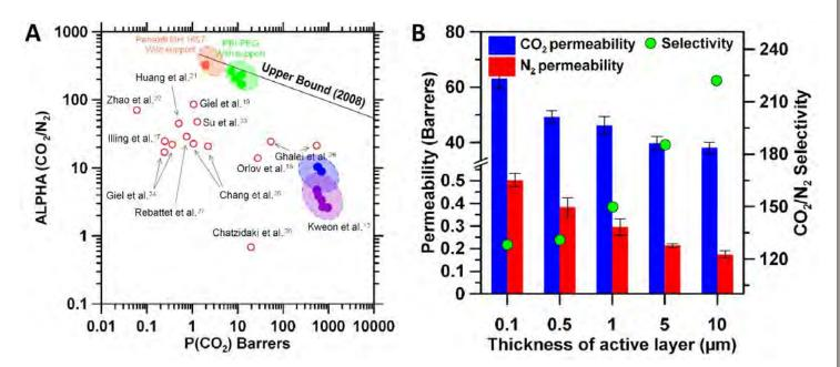
Figure 2: (A) A Robeson plot comparing the performance of the developed HypoMem against other polymer composite membranes for CO<sub>2</sub>/N<sub>2</sub> gas separations. (B) Permeability and ideal selectivity data for different thicknesses of active layers with pure CO<sub>2</sub> and N<sub>2</sub>.
