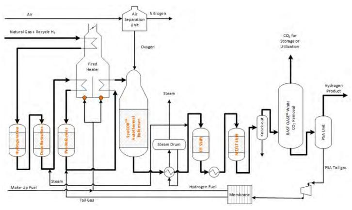
Figure 3: Process concept for integrated ATR with CO<sub>2</sub> capture.
