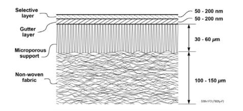
Figure 4: Schematic of TFC membranes comprising a selective layer, gutter layer, and porous support.
