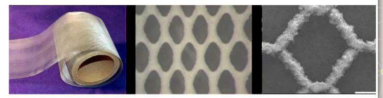
Figure 1: Microlith® mesh coated with sorbent.
