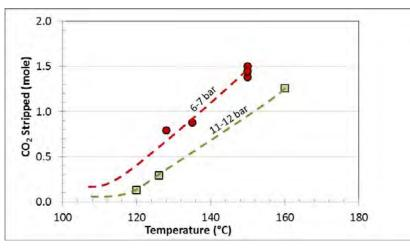
Figure 6: CO<sub>2</sub> stripping as a function of regeneration temperature and pressure.
