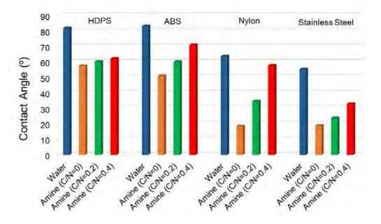
Figure 2: Contact angle of water and aqueous amines (at different CO<sub>2</sub> loadings) on different packing material surfaces.
