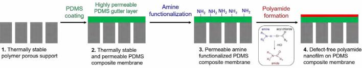
Figure 1: Preparation steps for a cross-linked polyamide nanofilm on a PDMS composite membrane.
