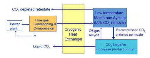
Figure 1: Block diagram of the cold membrane process.
