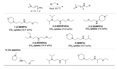
Figure 1: Selected library for non-volatile, low-viscosity secondary/tertiary diamines.
