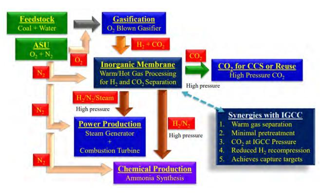
Figure 1: Inorganic membrane technology role in polygeneration cycle.
