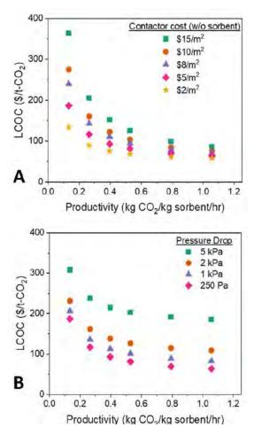
Figure 2: Pre-screen TEA results. Levelized cost of CO<sub>2</sub> capture as a function of productivity and (A) contactor cost or (B) pressure drop. Other parameters are held constant, including one-year sorbent lifetime, -65 kJ/mol heat of adsorption, 300 seconds cycle time, and 100,000 tonne CO<sub>2</sub>/year captured.
