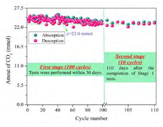
Figure 2: Demonstration of stability of MEA/(EMmim<sup>+</sup>)(NTF<sup>2-</sup>) CO<sub>2</sub> capture system in cyclic CO<sub>2</sub> absorption-desorption tests for more than five months.
