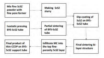
Figure 5: Tubular CCDP membrane fabrication.
