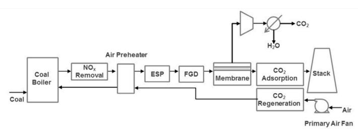
Figure 1: Flow diagram of the TDA Research hybrid membrane-sorbent CO<sub>2</sub> capture system.
