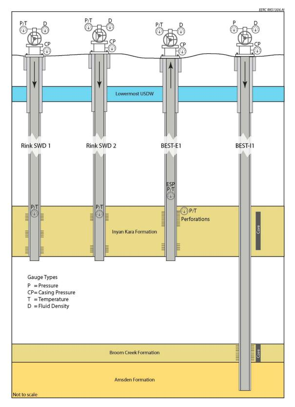
Figure 9-1. Schematic illustrating the active reservoir monitoring systems proposed for the BEST-E1, BEST-I1, Rink SWD 1, and Rink SWD 2 wells.
