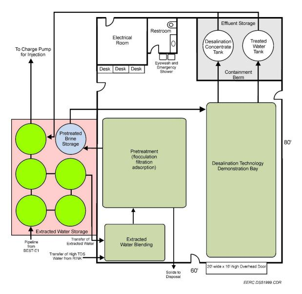
Figure 11-1. Johnsons Corner treatment technology test bed layout.
