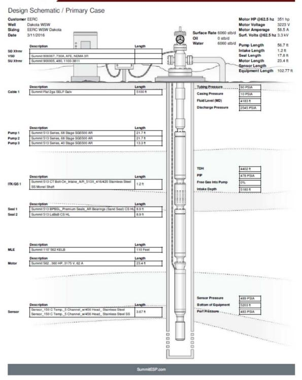
Figure D-19. Design schematic for Summit ESP assembly provided by Summit.
