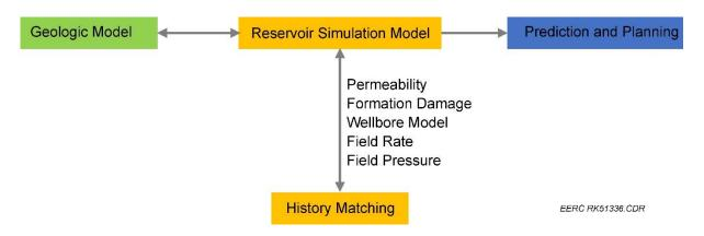
Figure A-15. Workflow for reservoir simulation, history matching, and prediction.
