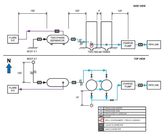
Figure 10-7. Engineering schematic of BEST-E1 facilities showing the location of major equipment and the process flow diagram between the wellhead and pipeline.
