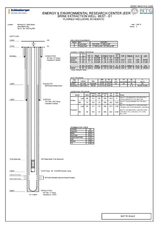
Figure 10-5. BEST-E1 well schematic.
