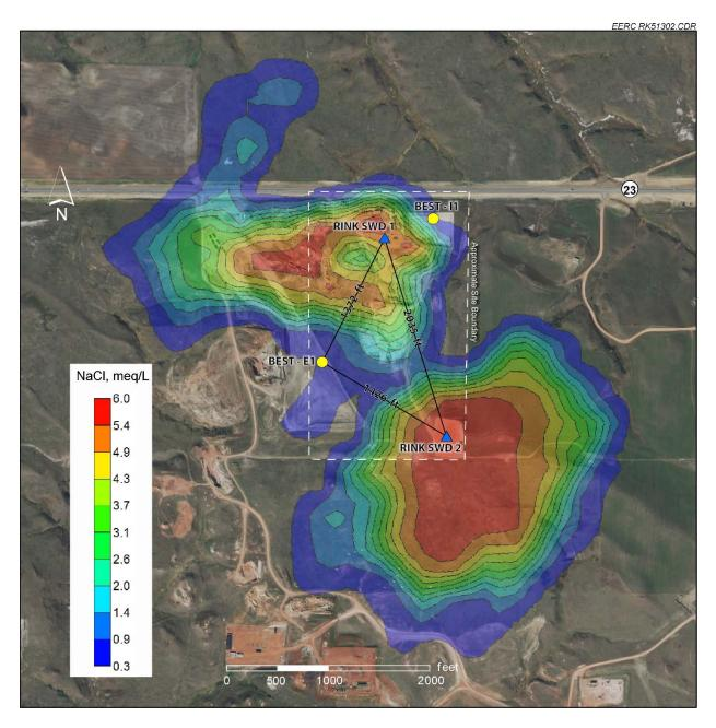
Figure 6-3. Distribution of the salinity plume on 1 April 2017 (as determined by simulation, within the Inyan Kara Formation superimposed over a site map). Proposed project wells are identified.
