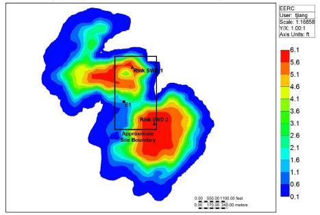
Figure 8-5. Salinity (molar concentration) of plume development in January 2020 without brine extraction, business as usual (above), and with the extraction experimental scenario (below). Note the significantly reduced footprint of the plume on the southwest side of the site.
