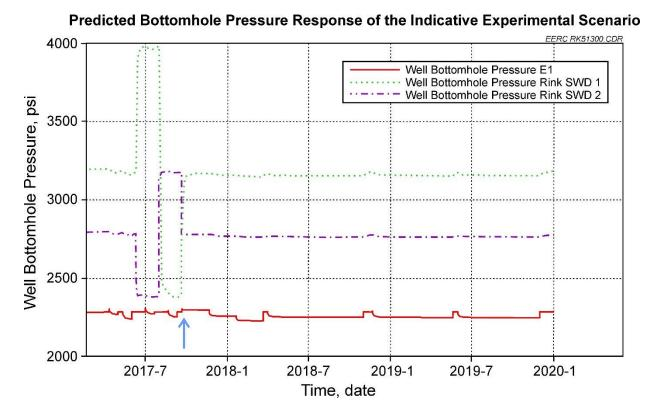
Figure 8-2. BHP response of the wells during the entire project experimental scenario. The end of interference testing and Stage 1 is indicated by the blue arrow. Changes in pressure responses of Rink SWD 1 and 2 to changing test parameters are visible throughout the experimental run.
