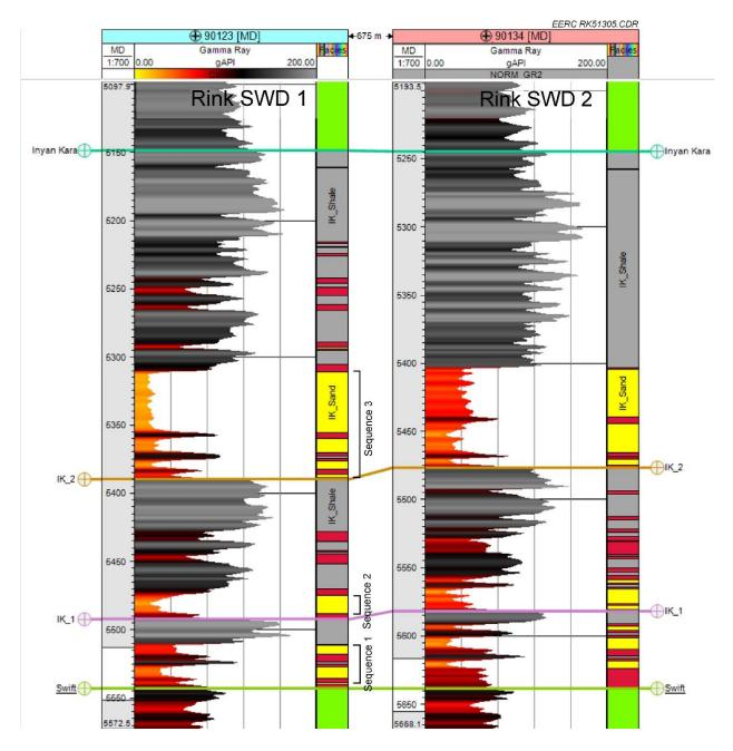
Figure 5-2. Correlation of injection wells Rink SWD 1 (left) and Rink SWD 2 (right). Curves shown for each well are GR and a facies log. The Inyan Kara Formation is split into three fining upward sequences.
