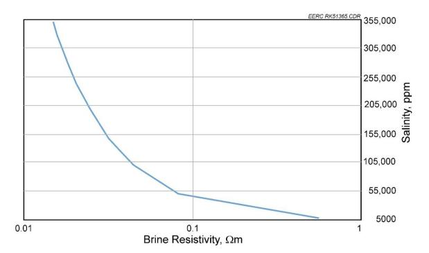
Figure A-41. Plots of brine salinity versus brine resistivity (using Crain, 1986).
