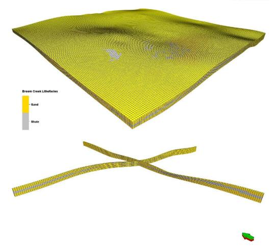
Figure 5-5. Facies distribution of the Broom Creek Formation portion of the model. The images illustrate the same full formation model view (top) and cross-section lines (bottom) as illustrated in Figure 5-4. Note that neither of the Rink SWD wells penetrates the Broom Creek, vertical exaggeration =  $10 \times$ .
