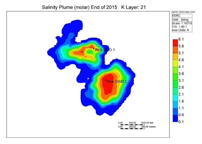
Figure A-20. Salinity plume development (molar concentration). Layer 21 indicates the maximum areal extent at the end of year 2015.
