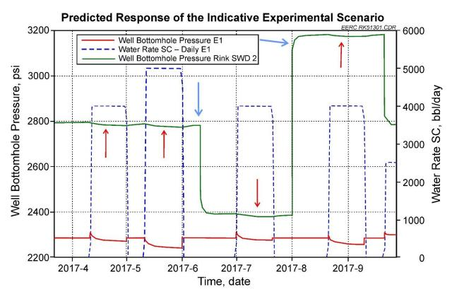
Figure 8-1. Predicted pressure response of the Rink SWD 2 well to changes in extraction rate. Changes in BHP due to changing injection rates are clearly visible (indicated by blue arrows). However, subtle dips in the BHP of Rink SWD 2 also occur in response to fluid extraction from the BEST-E1 well (indicated by red arrows).
