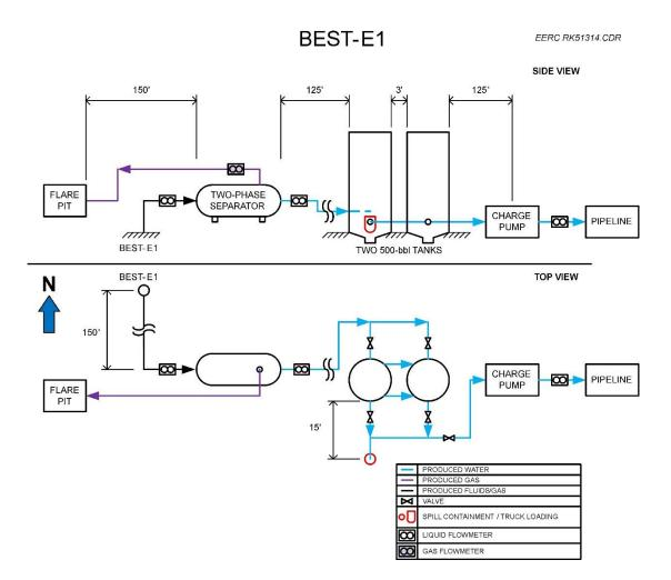
Figure D-18. BEST-E1 engineered drawings of flow path.
