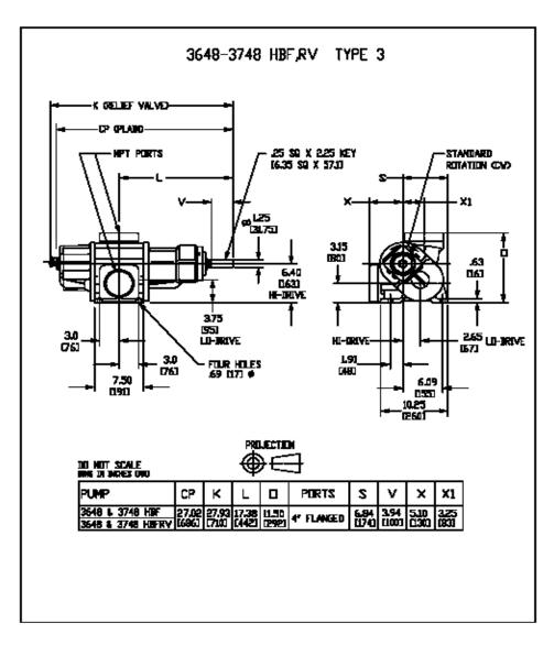
Figure D-31. Roper Pumps specification data sheet.
