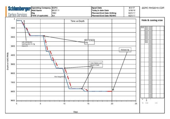
Figure D-1. Proposed time line for BEST-I1 well drilling provided by SLB.
