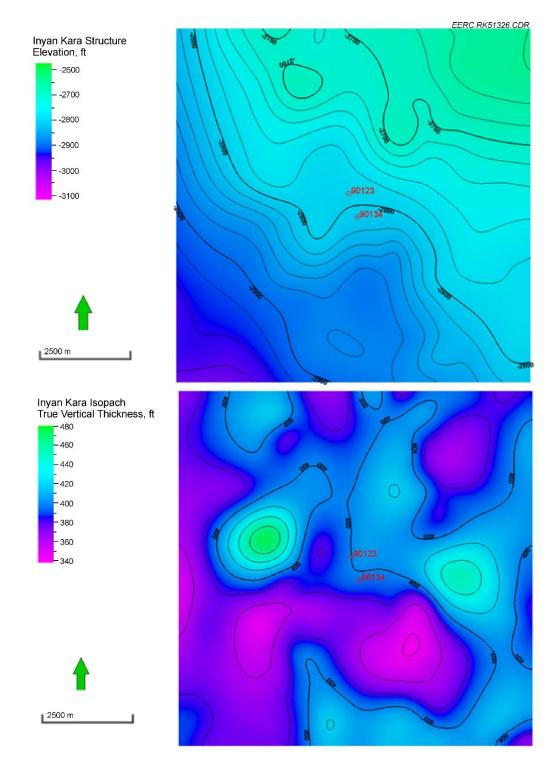
Figure A-4. Top: structure contour map on top of the Inyan Kara Formation within the Johnsons Corner study area. Datum: mean sea level. Bottom: isopach map of the Inyan Kara Formation within the Johnsons Corner study area. Injection Wells 90123 (Rink SWD 1) and 90134 (Rink SWD 2) are shown in red. Contour interval = 20 ft.
