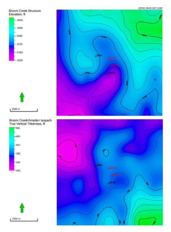
Figure A-5. Top: structure contour map on top of the Broom Creek Formation within the Johnsons Corner study area. Datum: mean sea level. Bottom: isopach map of the combined Broom Creek and Amsden Formations within the Johnsons Corner study area. Injection
