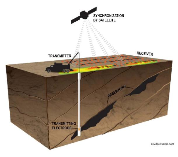
Figure A-43. Schematic from GroundMetrics, a BSEM provider, shows the survey geometry with a downhole electrode, surface transmitter, and surface receiver array synchronized by GPS satellite (courtesy GroundMetrics).
