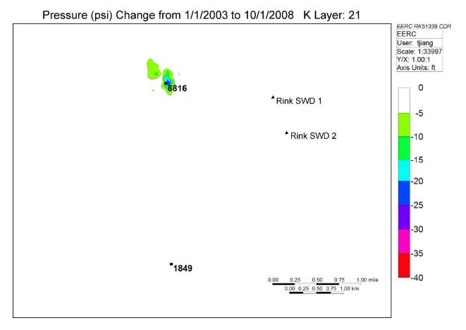
Figure A-18. Pressure difference map from January 1, 2003, to October 1, 2008, illustrating the maximum pressure differential resulting from Well 8816.
