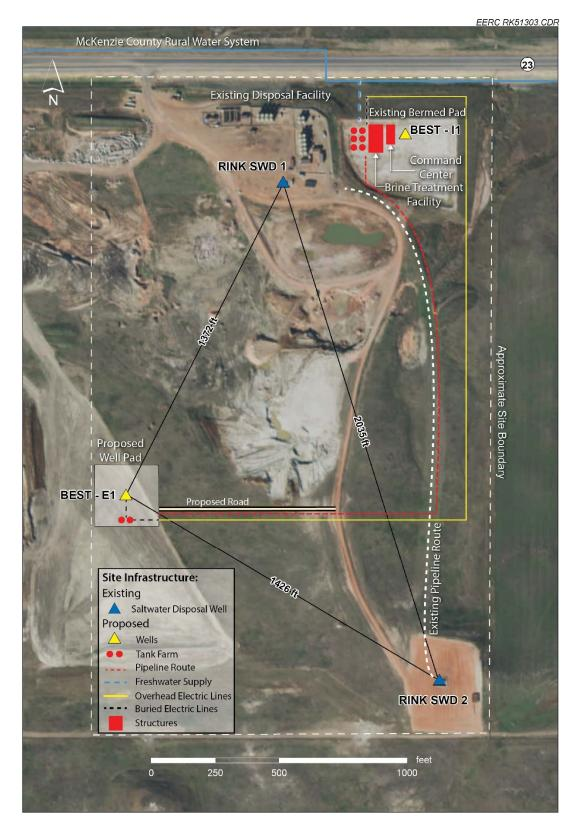
Figure A-25. Selected well locations for Johnsons Corner project execution and placement of associated new infrastructure.
