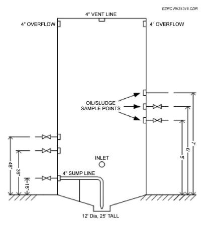
Figure D-9. Individual 500-bbl fiberglass tank schematic.
