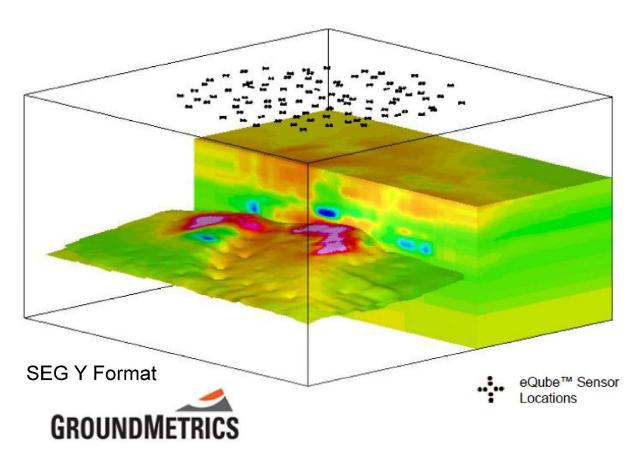
Figure A-45. Resistivity volume deliverable in SEGY format ready for interpretation (courtesy GroundMetrics).
