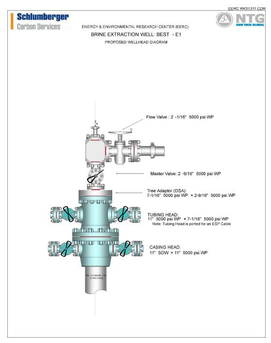
Figure D-17. BEST-E1 wellhead schematic provided by SLB.
