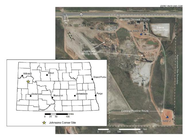
Figure 4-1. Aerial image of the Johnsons Corner site located in McKenzie County, North Dakota, highlighting the location of existing mining, lease roads, brine-handling facilities, pipeline, prepared pad for permitted extracted brine treatment facilities, and the existing Rink SWD 1 and Rink SWD 2 wells.
