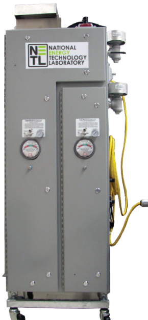
Raman gas analyzer field prototype.
