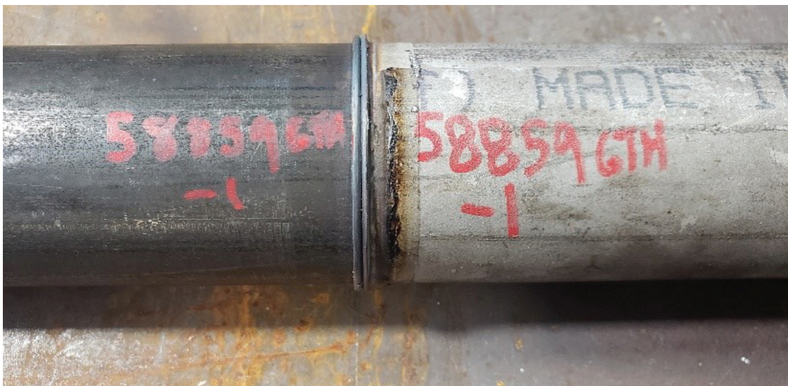
Rotary friction welded T91 to 304H tube.
