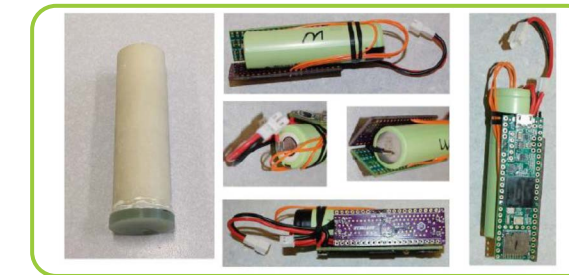
Visual Inspection of Sensor Prototype After Exposure Testing
