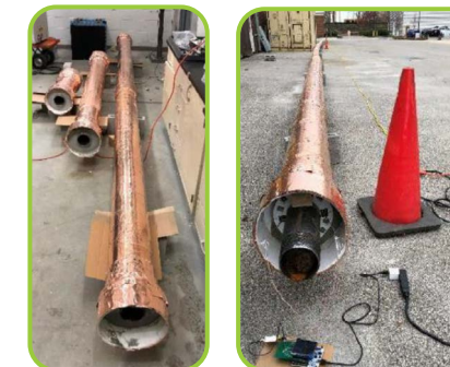
3- to 120-ft-Long Pipe-in-Pipe Set Up
