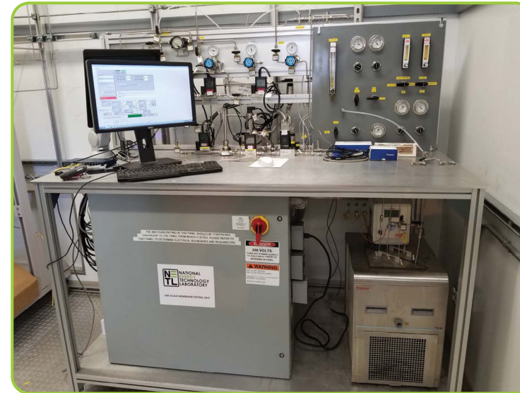
NETL's Membrane Test Unit at NCCC for Coal Flue Gas Decarbonization (Operational)
