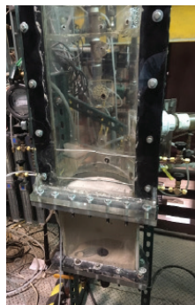
Semi-circular fluidized bed with side jets.
