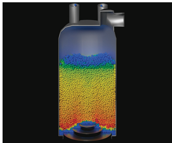
MFIX-DEM simulation of coal gasification in a 1 megawatt moving bed gasifier.
